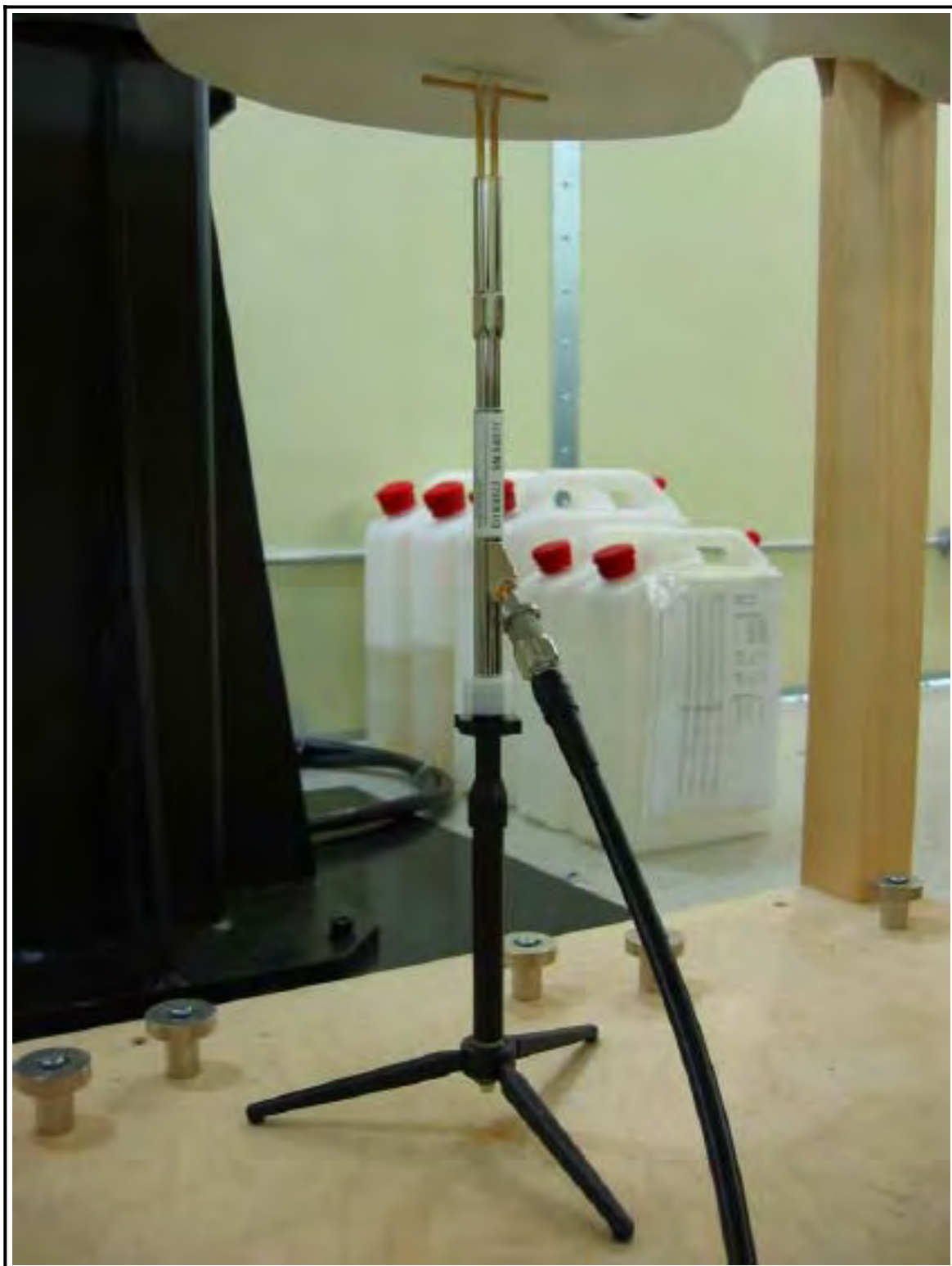
Figure 2 1900 MHz Dipole Validation Test Setup
