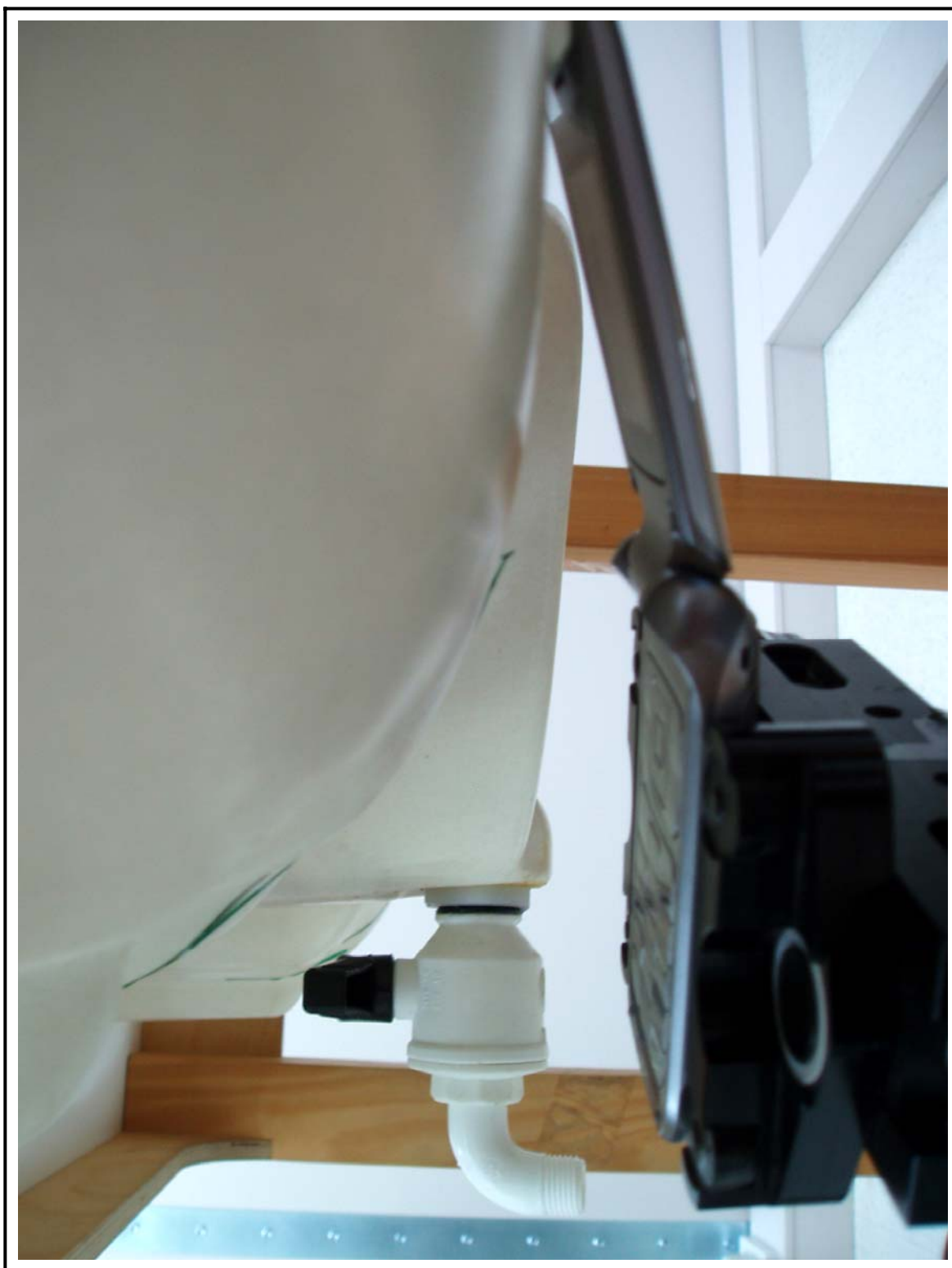
Figure 5 Left Head SAR Test Setup – Ear Tilt Position
