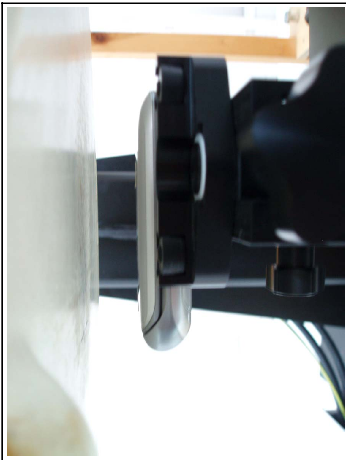
Figure 6 Body SAR Test Setup – w/o Holster
