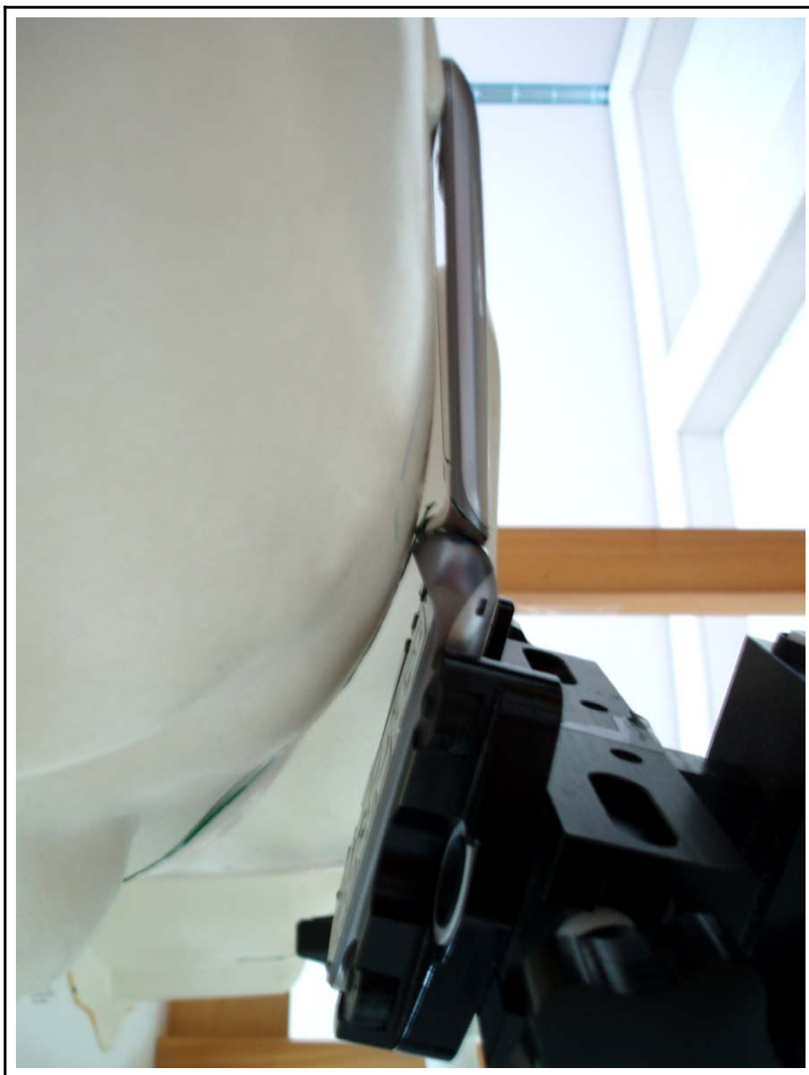
Figure 4 Left Head SAR Test Setup - Cheek Touch Position
