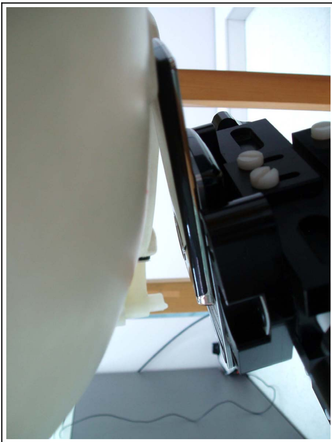
Figure 24 Left Head SAR Test Setup – Ear Tilt Position
