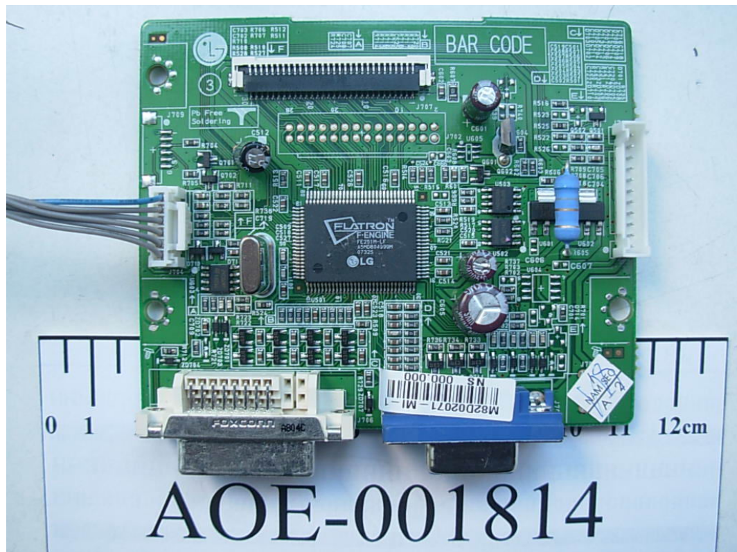
FIGURE 11 LCD MONITOR (M/N: L1742TT) MAIN BOARD (COMPONENT SIDE)
