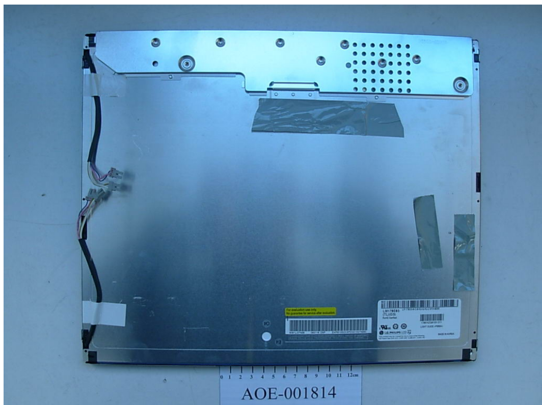
FIGURE 3 LCD MONITOR (M/N: L1742TT) LCD PANEL (BACK VIEW)
