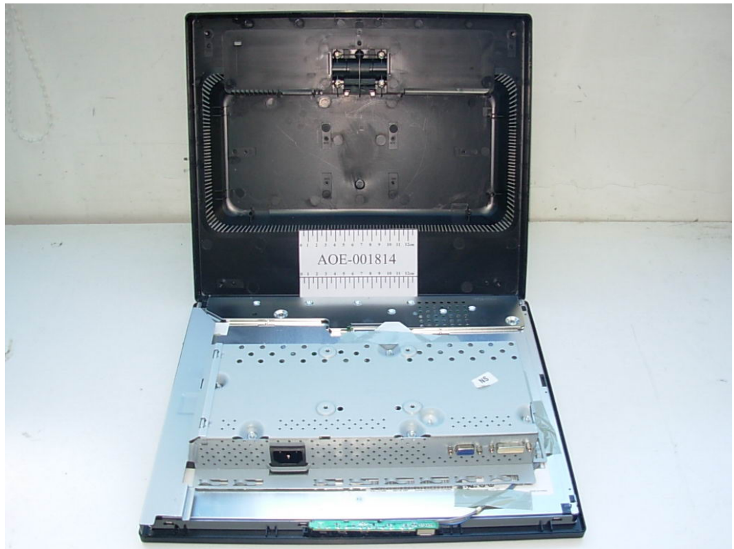
FIGURE 1 LCD MONITOR (M/N: L1742TT) COVER REMOVED
