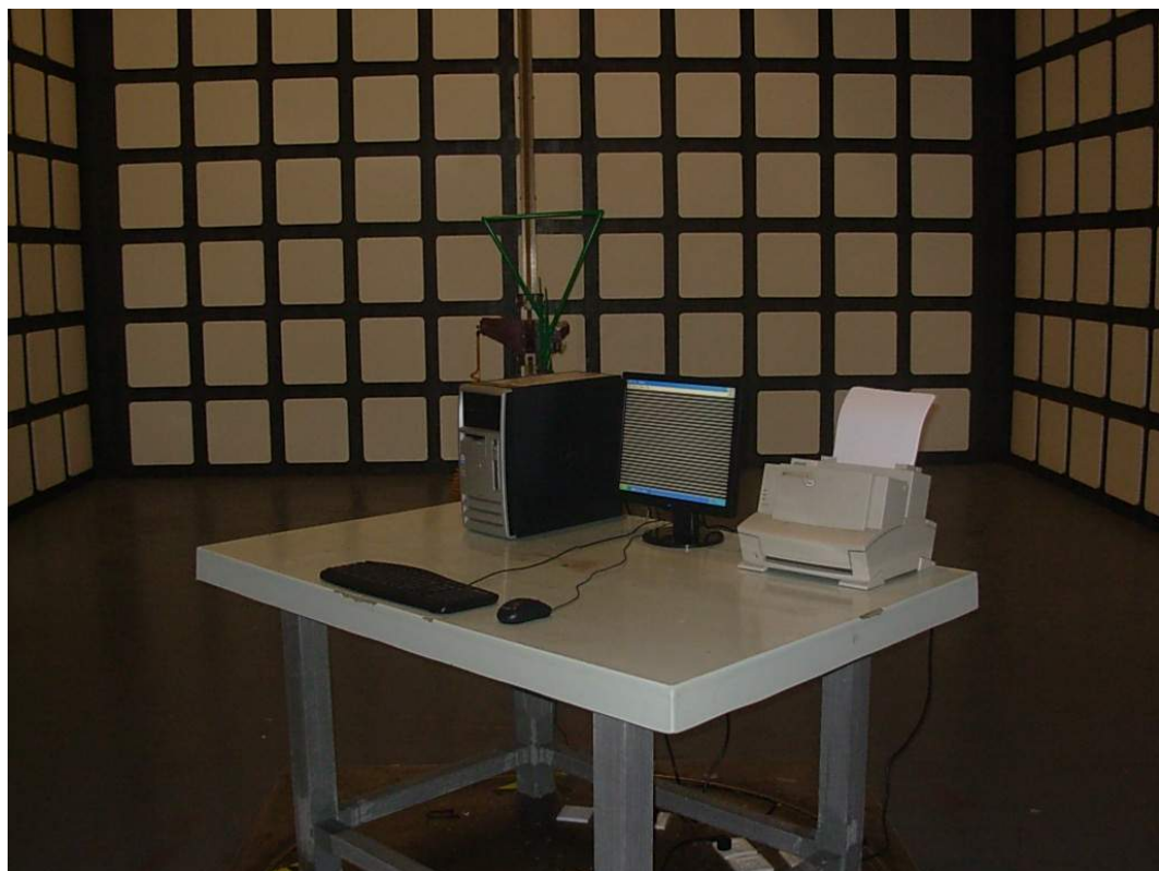
SETUP WITH MAXIMUM DETECTED EMISSION AT VERTICAL POLARIZATION (VGA 640*480@60Hz)
