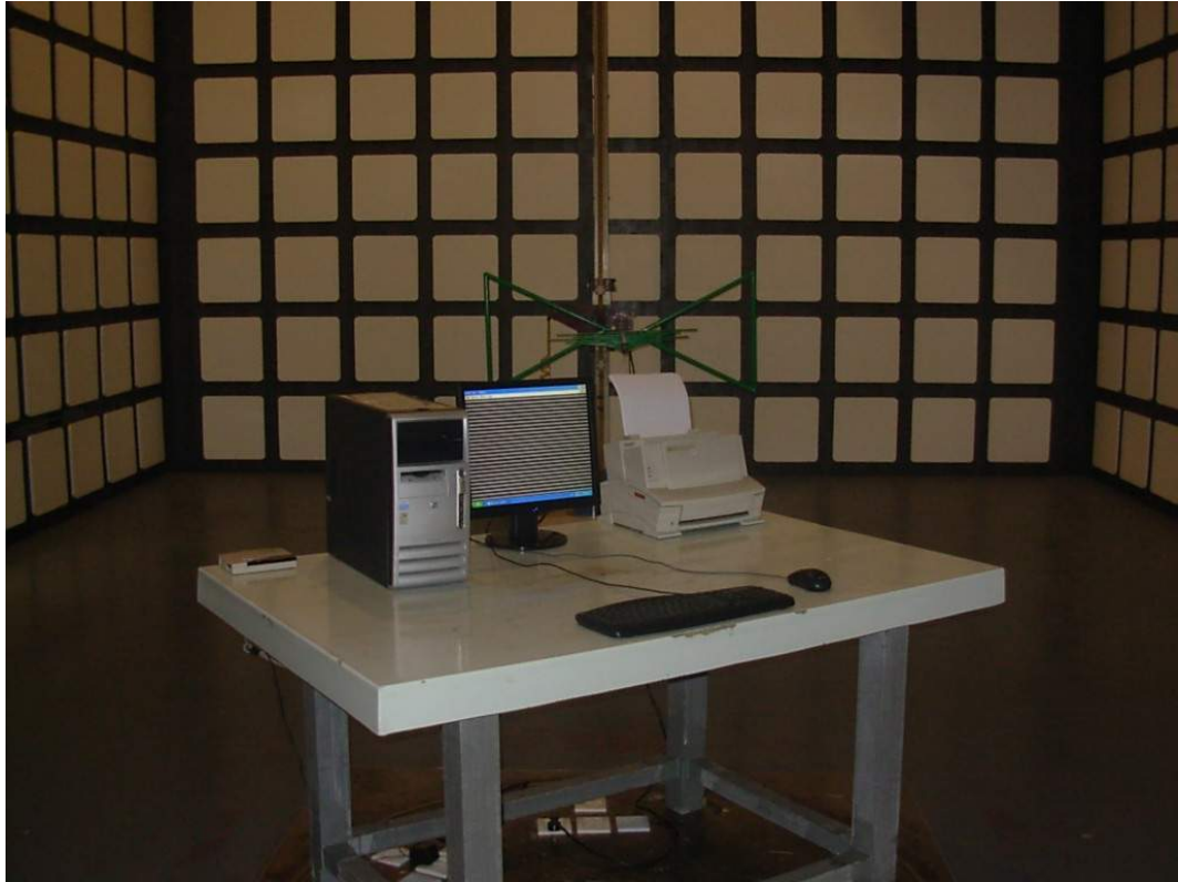
SETUP WITH MAXIMUM DETECTED EMISSION AT HORIZONTAL POLARIZATION (VGA 640*480@60Hz)
