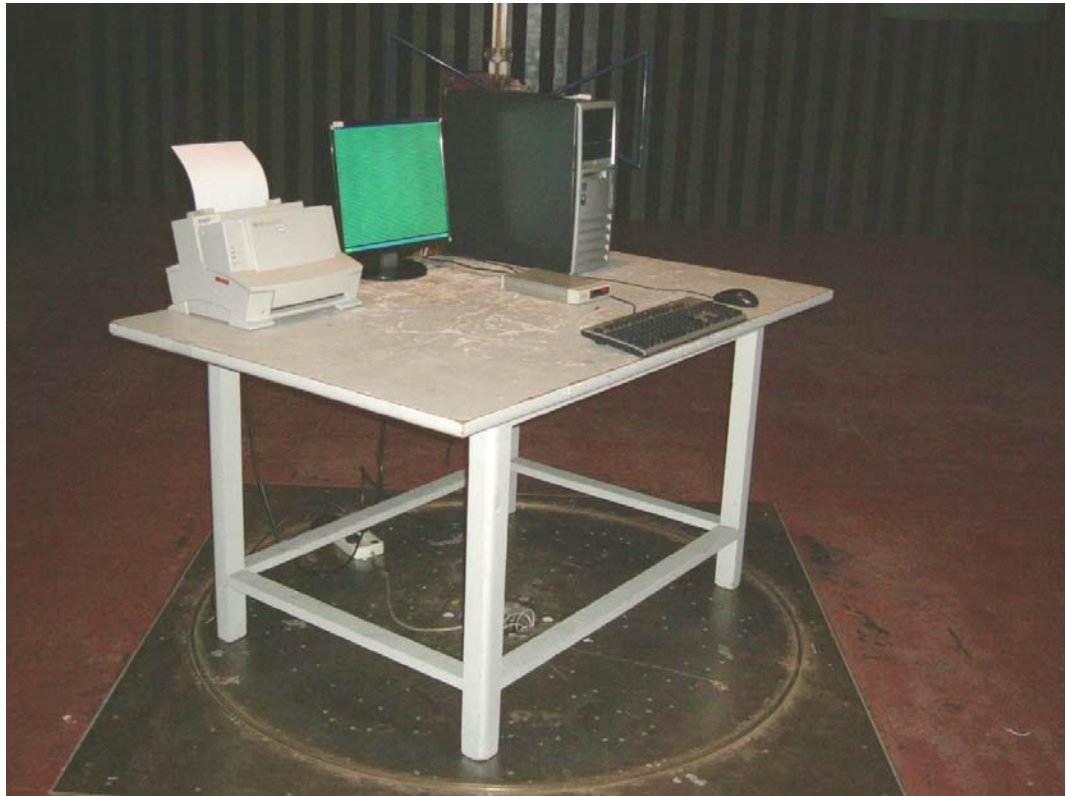
SETUP WITH MAXIMUM DETECTED EMISSION AT HORIZONTAL POLARIZATION (VGA 1024*768@75Hz)
