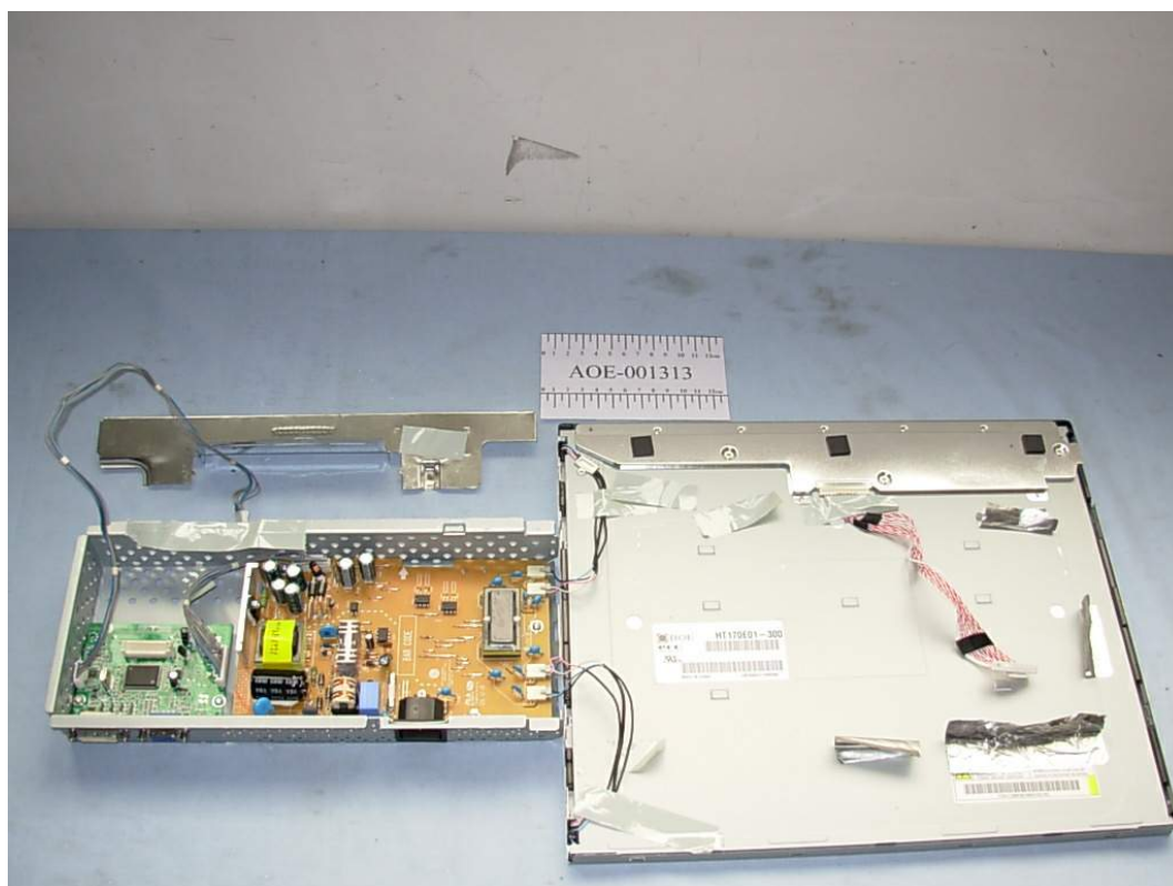
FIGURE 2 LCD MONITOR (M/N: L1753TS) SHIELDED COVER REMOVED
