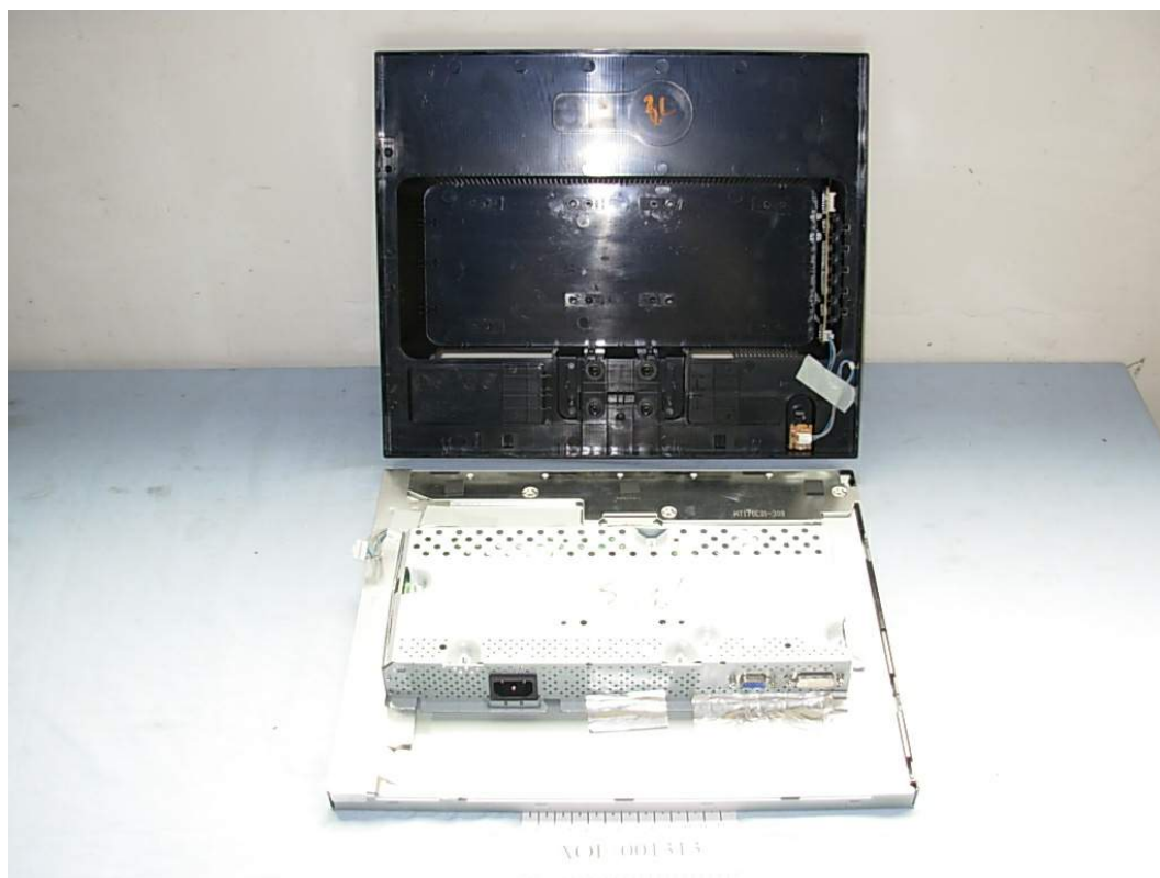
FIGURE 2 LCD MONITOR (M/N: L1753TS) SHIELDED COVER REMOVED
