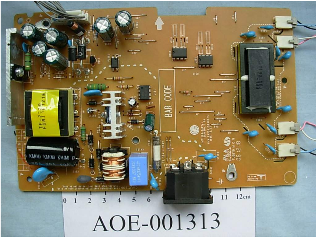
FIGURE 7 LCD MONITOR (M/N: L1753TS) POWER BOARD (COMPONENT SIDE)
