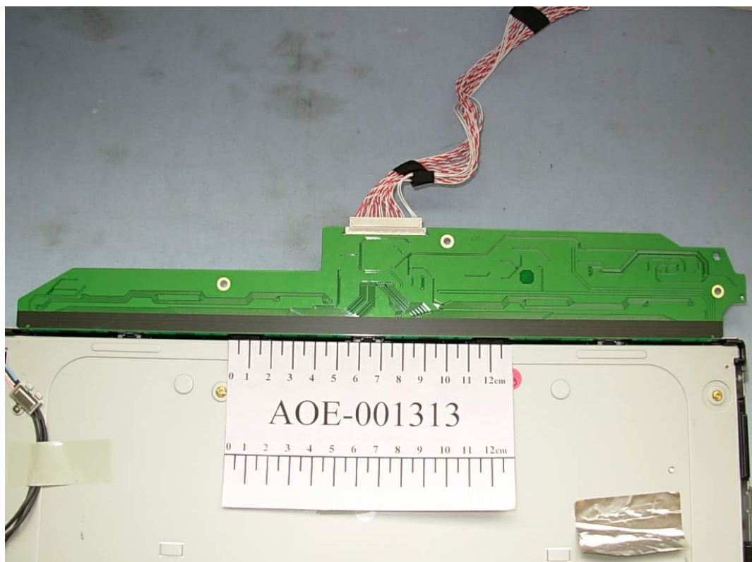
FIGURE 12 LCD MONITOR (M/N: L1753TS) LCD PANEL MAIN BOARD (SOLDERED SIDE)
