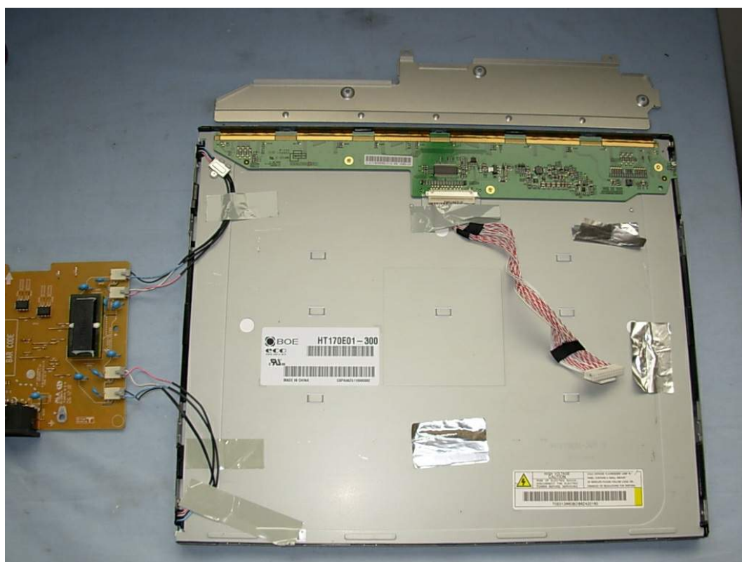
Figure 10 LCD MONITOR (M/N: L1753TS) LCD PANEL SHIELDED SHELL REMOVED
