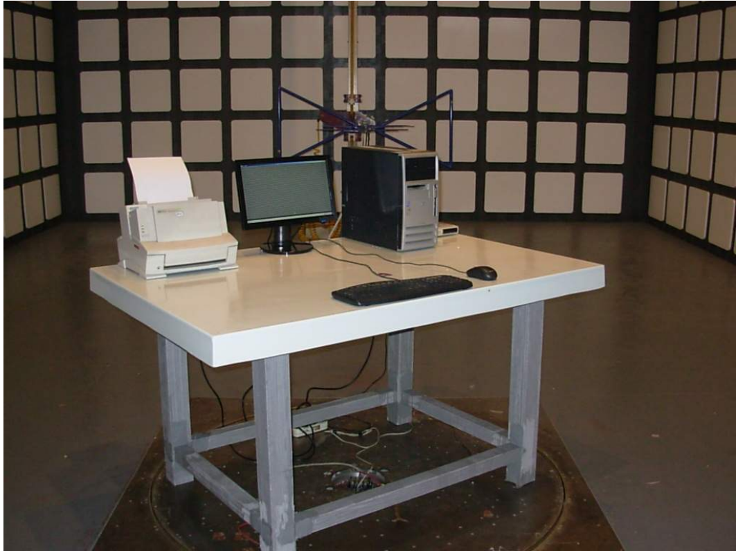
SETUP WITH MAXIMUM DETECTED EMISSION AT HORIZONTAL POLARIZATION (VGA 1024*768@60Hz, LOW FREQUENCY)
