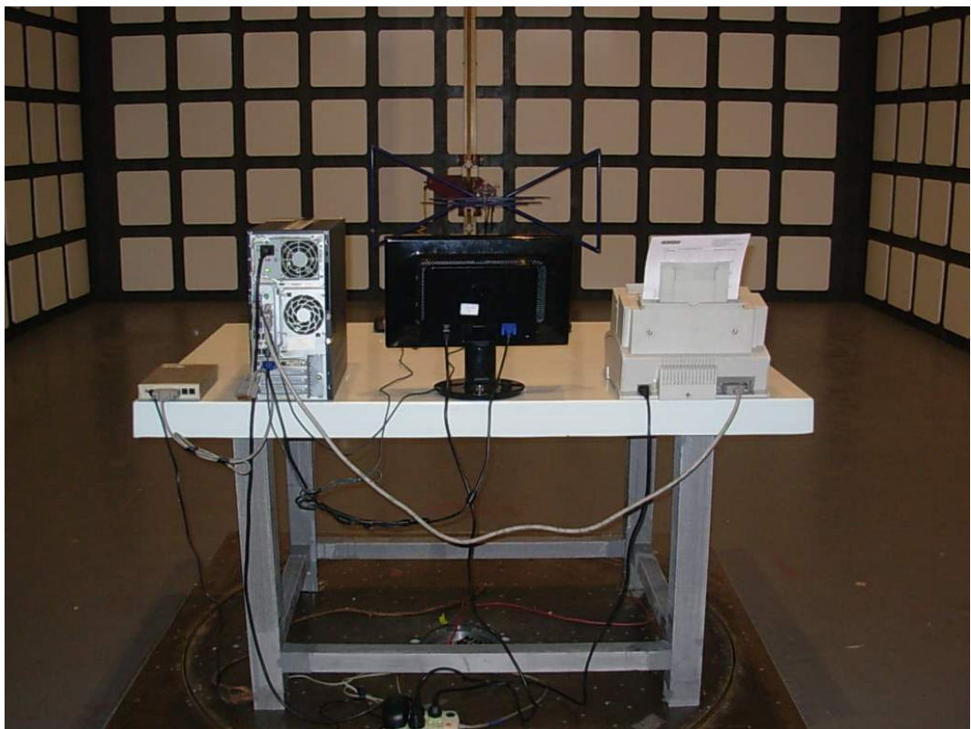
BACK VIEW OF RADIATED EMISSION TEST (LOW FREQUENCY)
