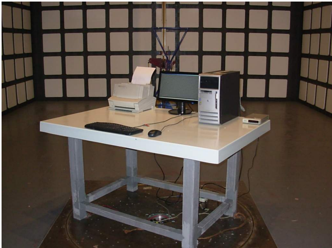
SETUP WITH MAXIMUM DETECTED EMISSION AT VERTICAL POLARIZATION (VGA 1024*768@60Hz, LOW FREQUENCY)
