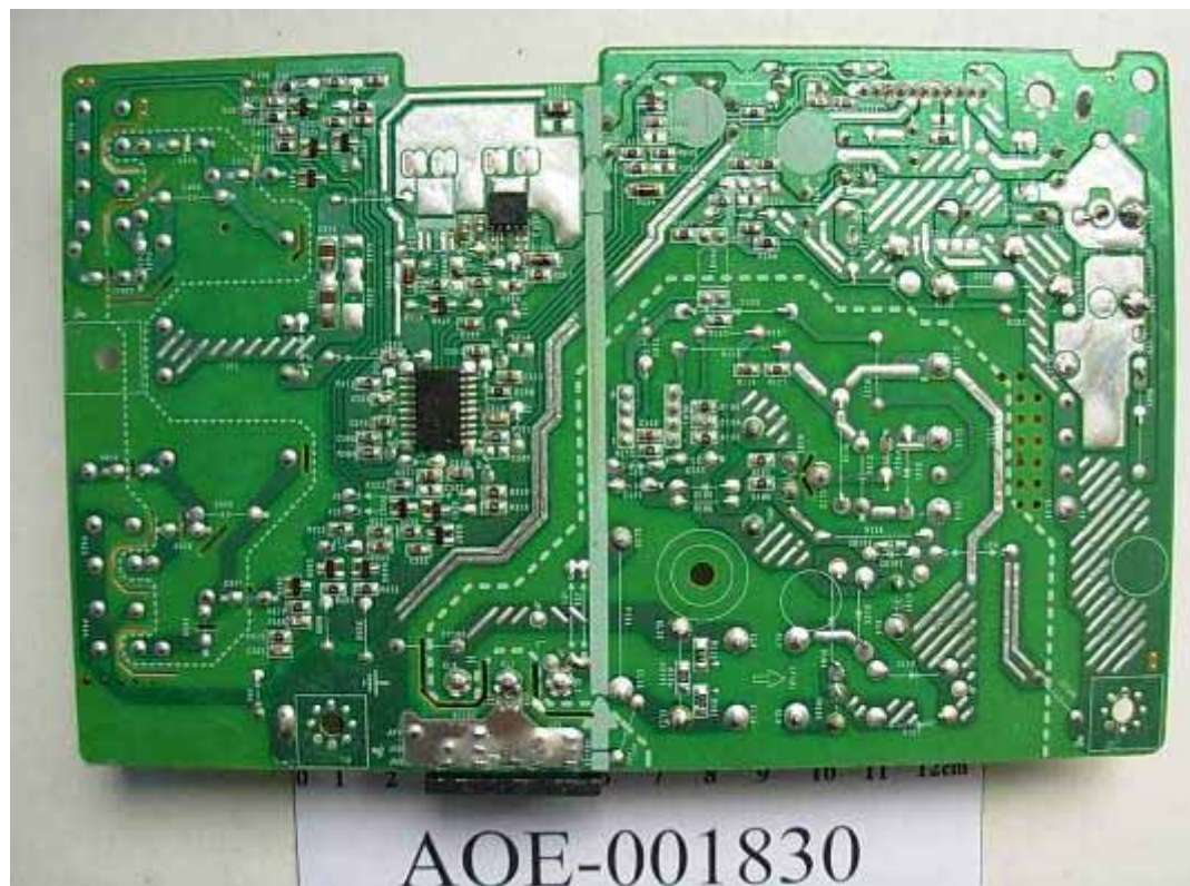
FIGURE 6 LCD MONITOR (M/N: L1942TT) POWER BOARD (SOLDERED SIDE)
