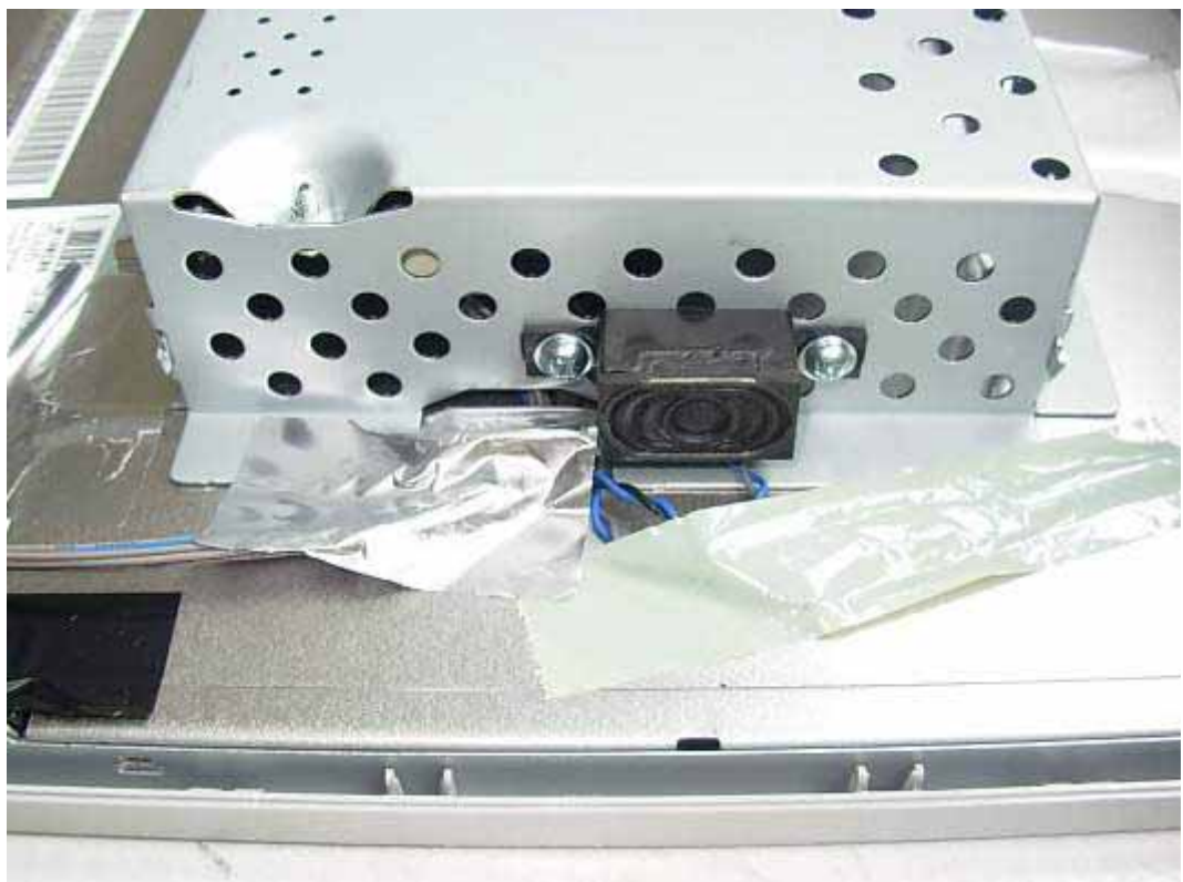
FIGURE 2 LCD MONITOR (M/N: L1942PKU) SPEAKER #1
