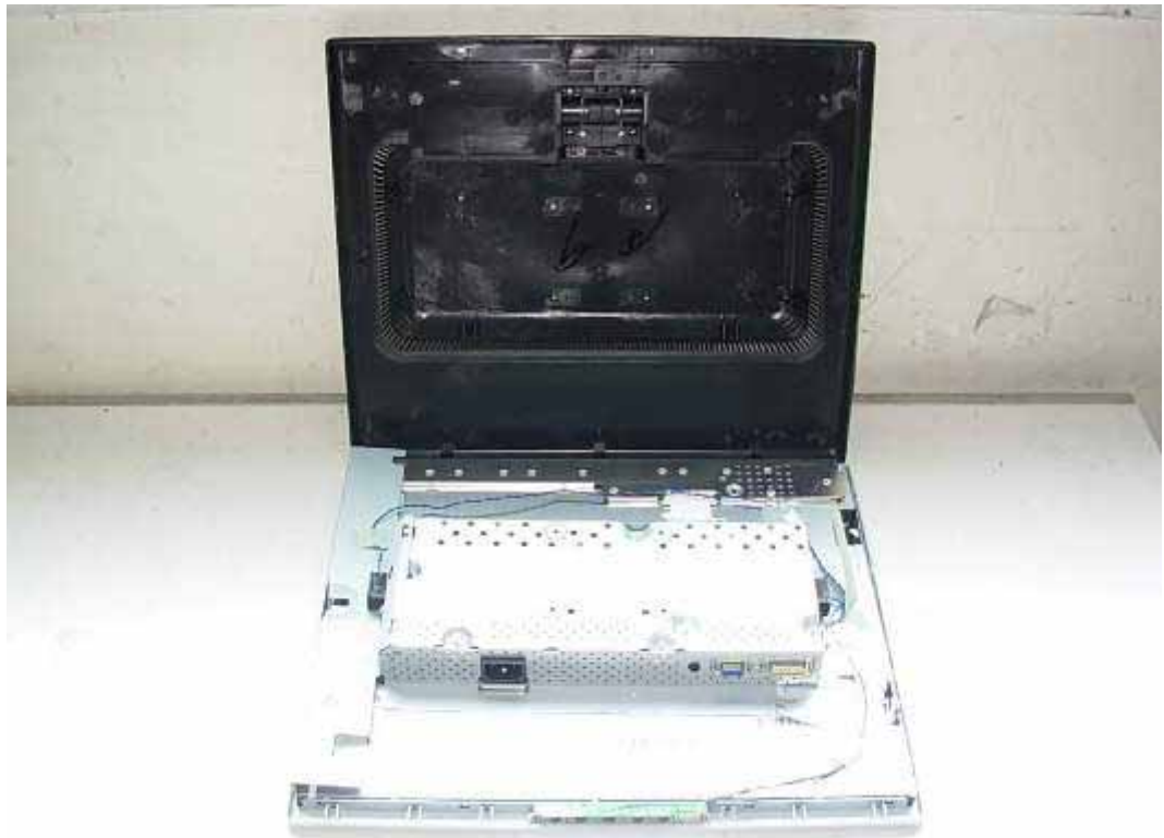
FIGURE 1 LCD MONITOR (M/N: L1942PKU) COVER REMOVED
