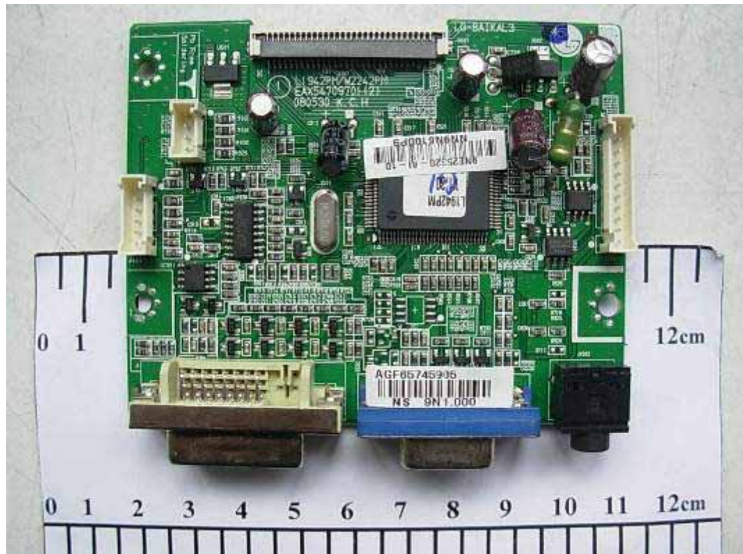
FIGURE 7 LCD MONITOR (M/N: L1942PKU) MAIN BOARD (COMPONENT SIDE)
