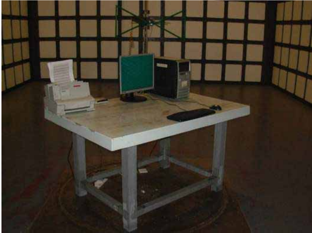
SETUP WITH MAXIMUM DETECTED EMISSION AT HORIZONTAL POLARIZATION (TEST MODE: DVI 1280*1024@60Hz)
