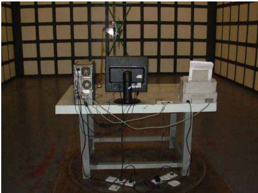
BACK VIEW OF RADIATED EMISSION TEST
