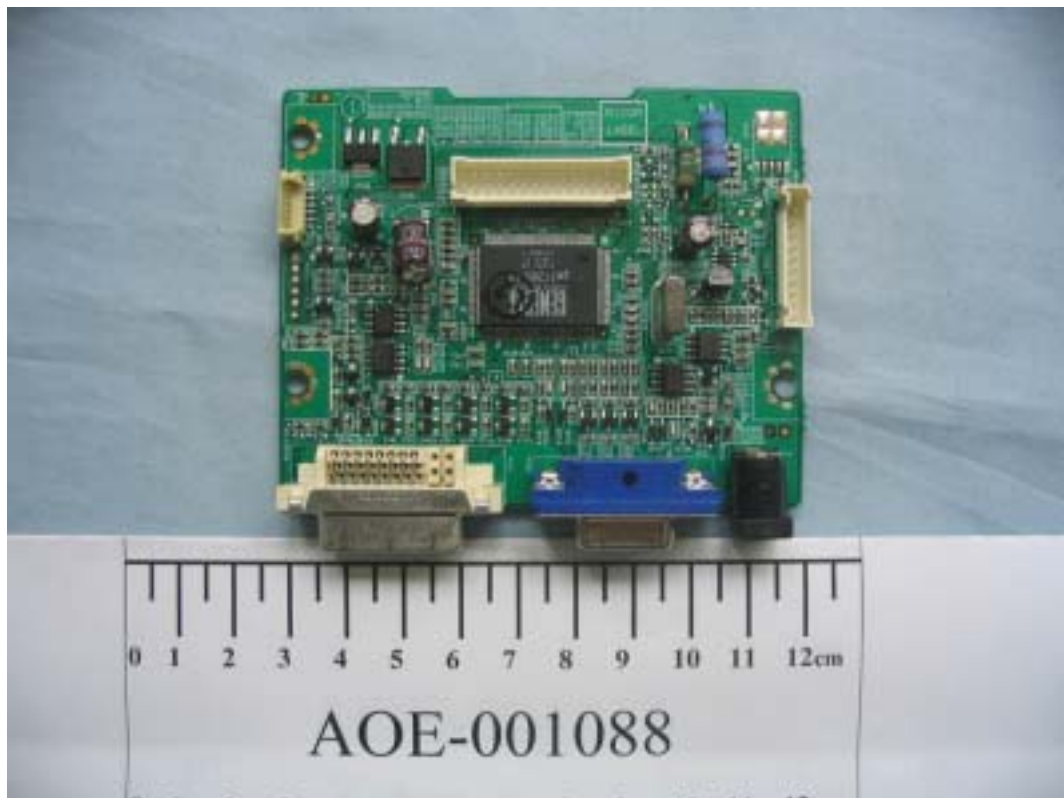
FIGURE 14 LCD MONITOR (M/N: L194WTM) MAIN BOARD (COMPONENT SIDE)
