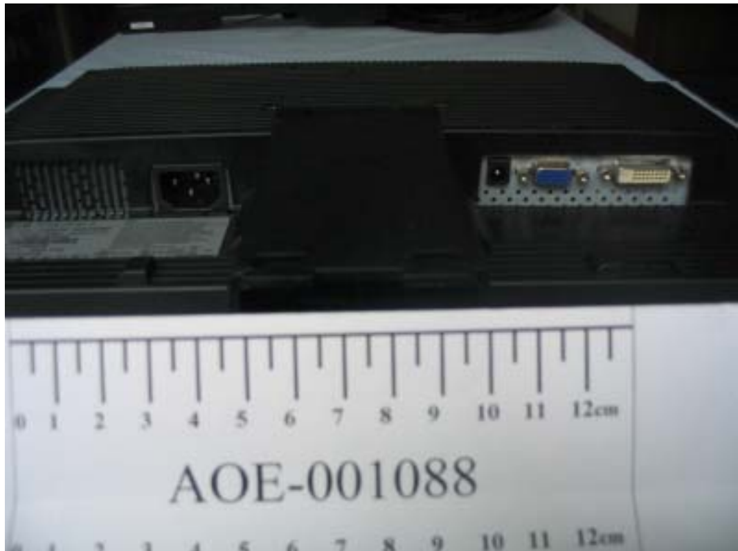
FIGURE 1 LCD MONITOR (M/N: L194WTM) PORTS VIEW
