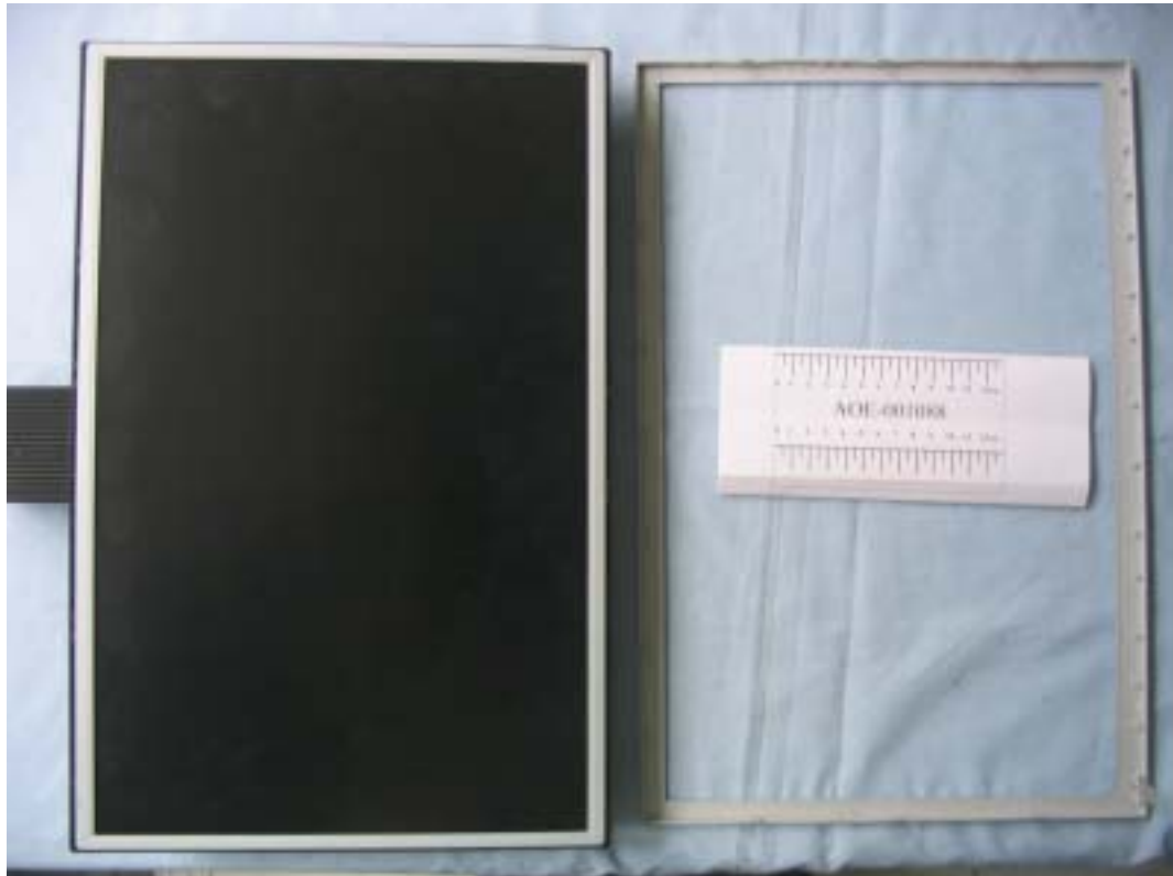
FIGURE 3 LCD MONITOR (M/N: L194WTM) FRONT COVER REMOVED
