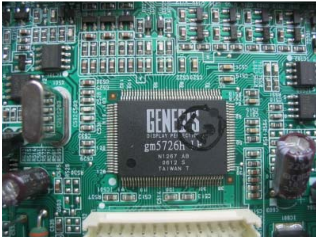
FIGURE 16 LCD MONITOR (M/N: L194WTM) MAIN BOARD - IC
