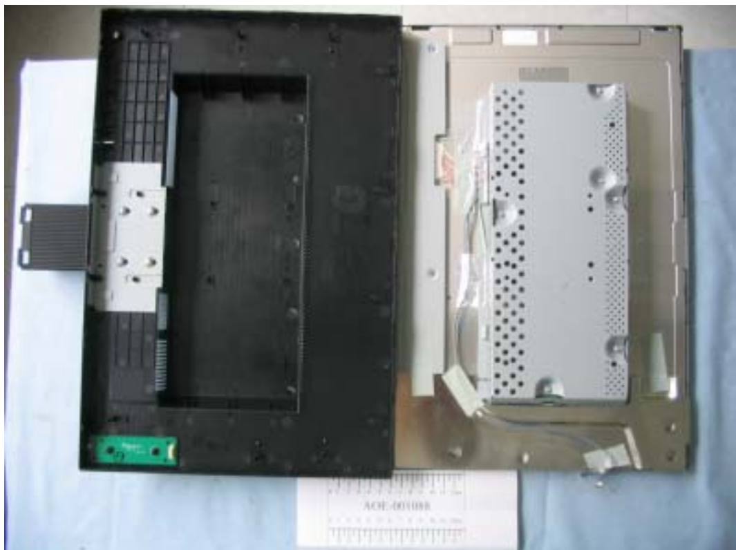
FIGURE 4 LCD MONITOR (M/N: L194WTM) REAR COVER REMOVED
