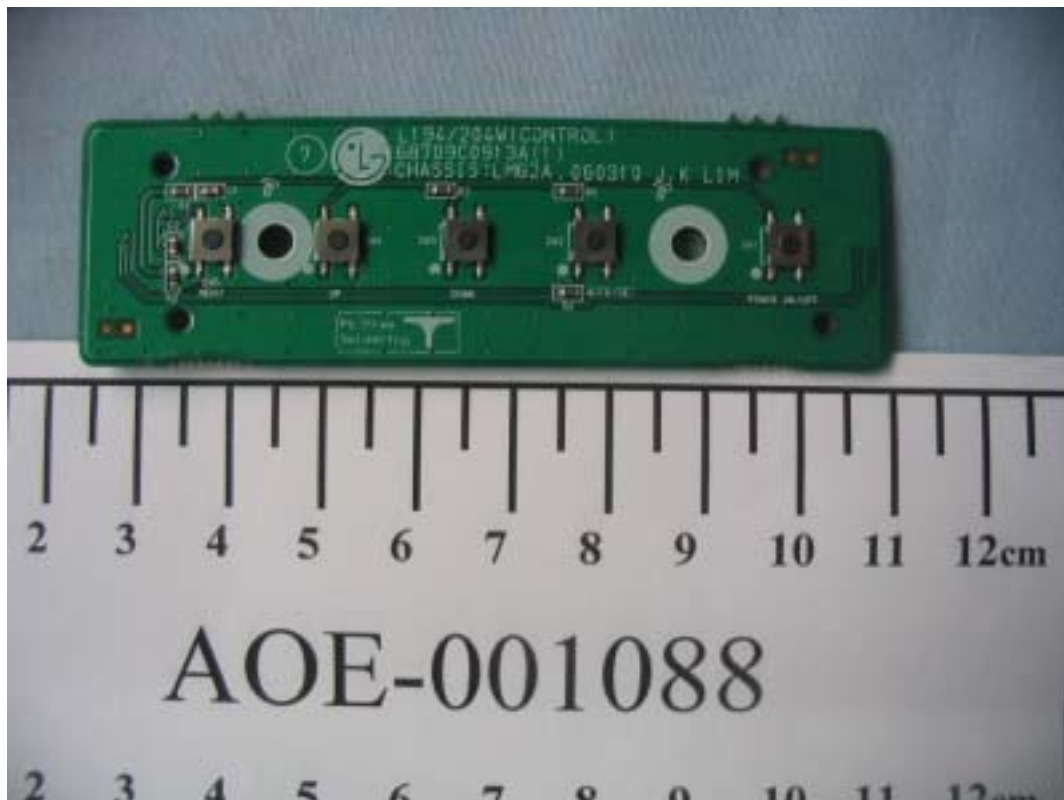
FIGURE 5 LCD MONITOR (M/N: L194WTM) CONTROL BOARD (COMPONENT SIDE)
