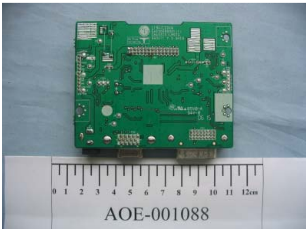
FIGURE 15 LCD MONITOR (M/N: L194WTM) MAIN BOARD (SOLDERED SIDE)
