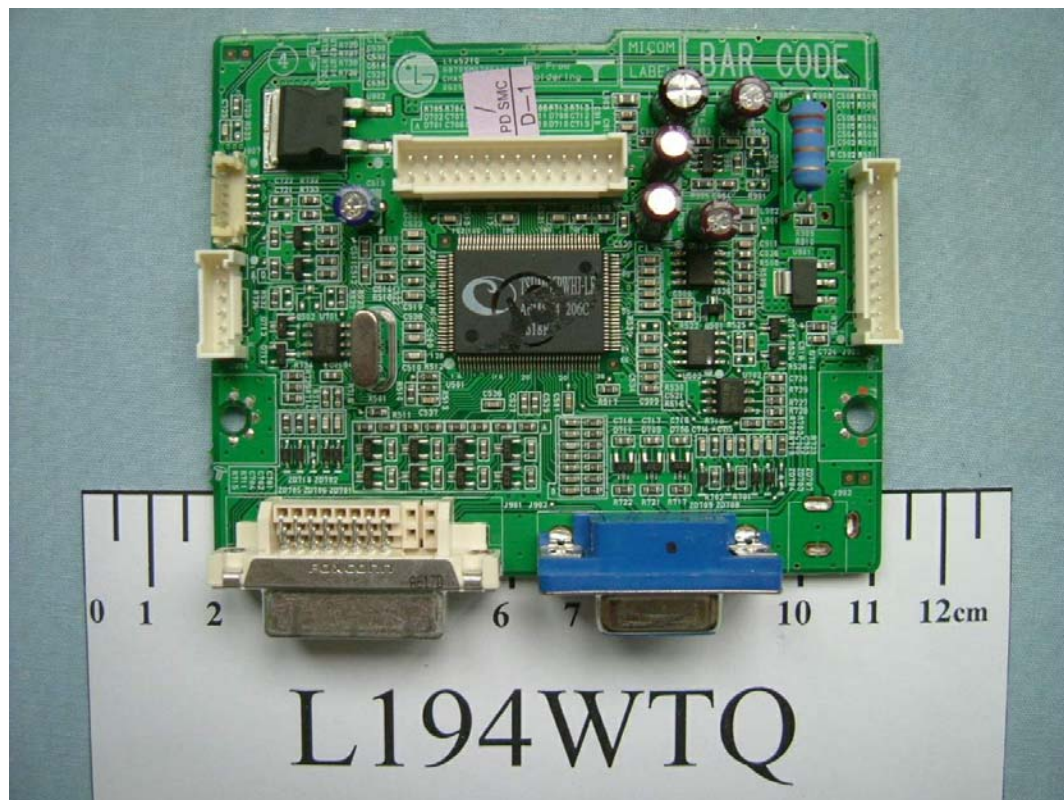
FIGURE 5 LCD MONITOR (M/N: L194WTQ) MAIN BOARD (COMPONENT SIDE)
