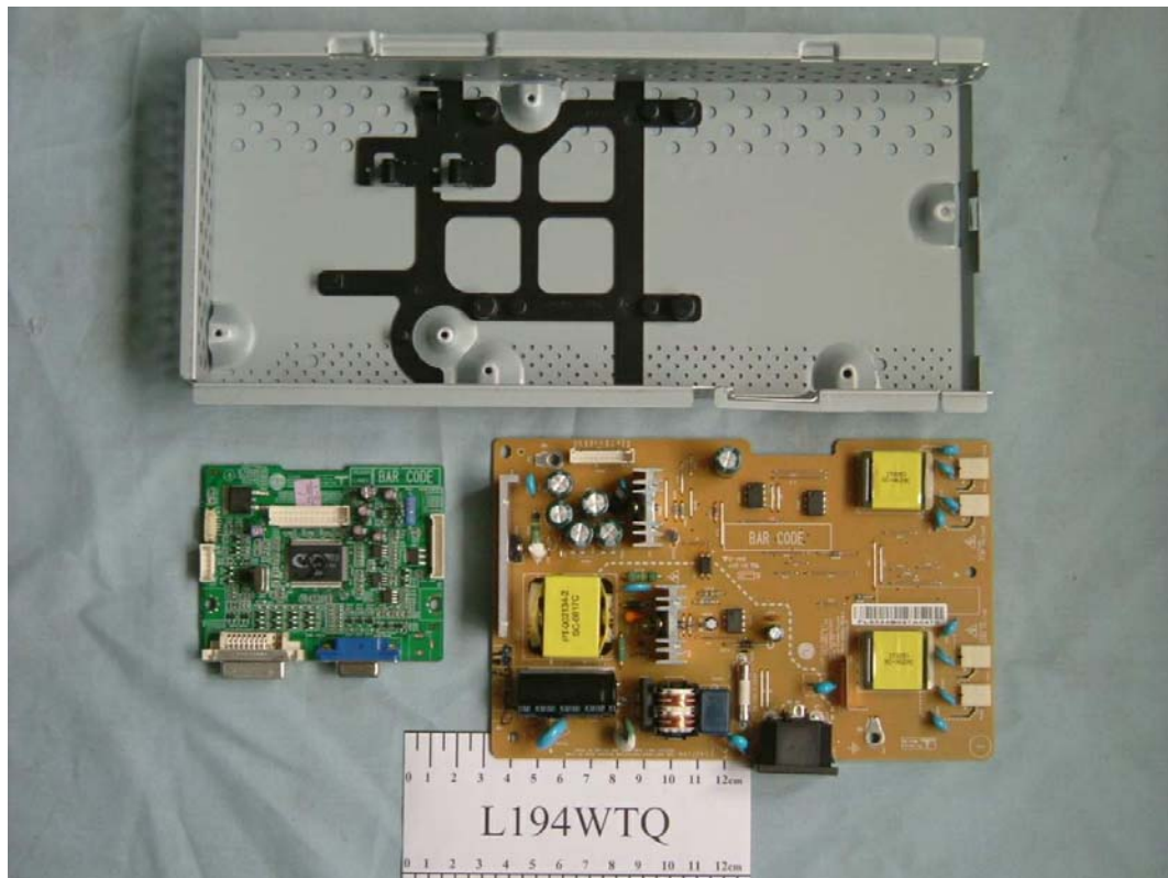
FIGURE 4 LCD MONITOR (M/N: L194WTQ) SHIELDED SHELL 2 REMOVED
