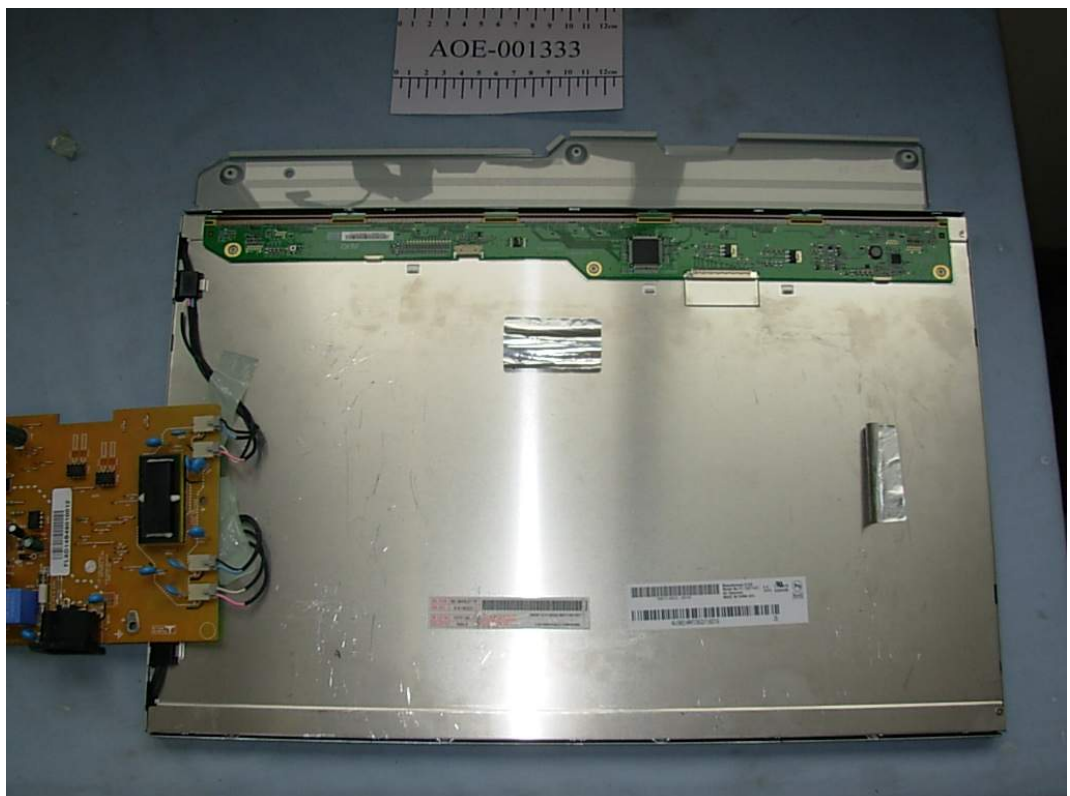
FIGURE 10 LCD MONITOR (M/N: L194WTS) LCD PANEL MAIN BOARD SHIELDED COVER REMOVED
