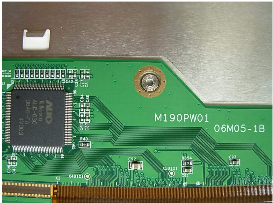
FIGURE 15 LCD MONITOR (M/N: L194WTS) CHIP & LABEL 1 ON LCD PANEL MAIN BOARD
