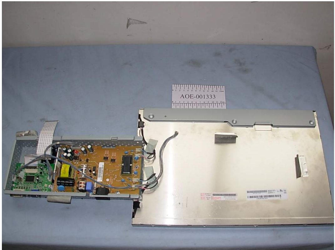
FIGURE 3 LCD MONITOR (M/N: L194WTS) BOARDS REMOVED
