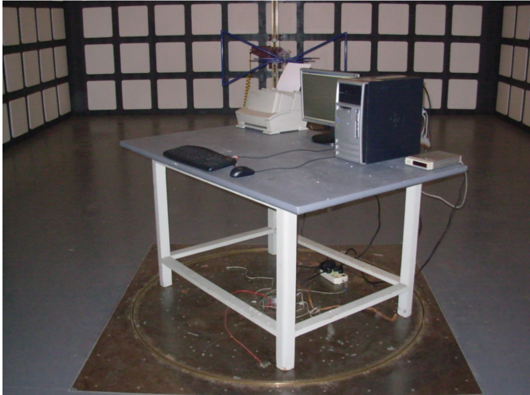
SETUP WITH MAXIMUM DETECTED EMISSION AT HORIZONTAL POLARIZATION (VGA 1440*900@60Hz)
