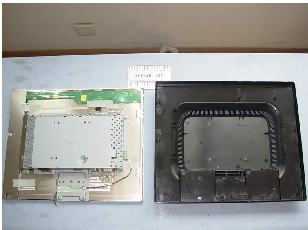
FIGURE 4 LCD MONITOR (M/N: L1954TS) COVER REMOVED
