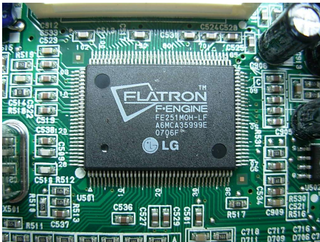
FIGURE 9 LCD MONITOR (M/N: L1954TS) CHIP ON MAIN BOARD
