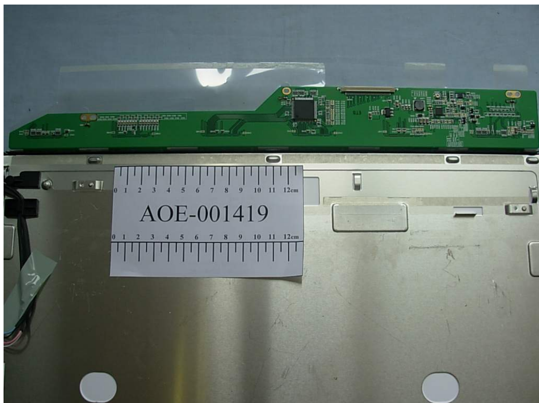
FIGURE 16 LCD MONITOR (M/N: L1954TS) LCD PANEL MAIN BOARD BACK
