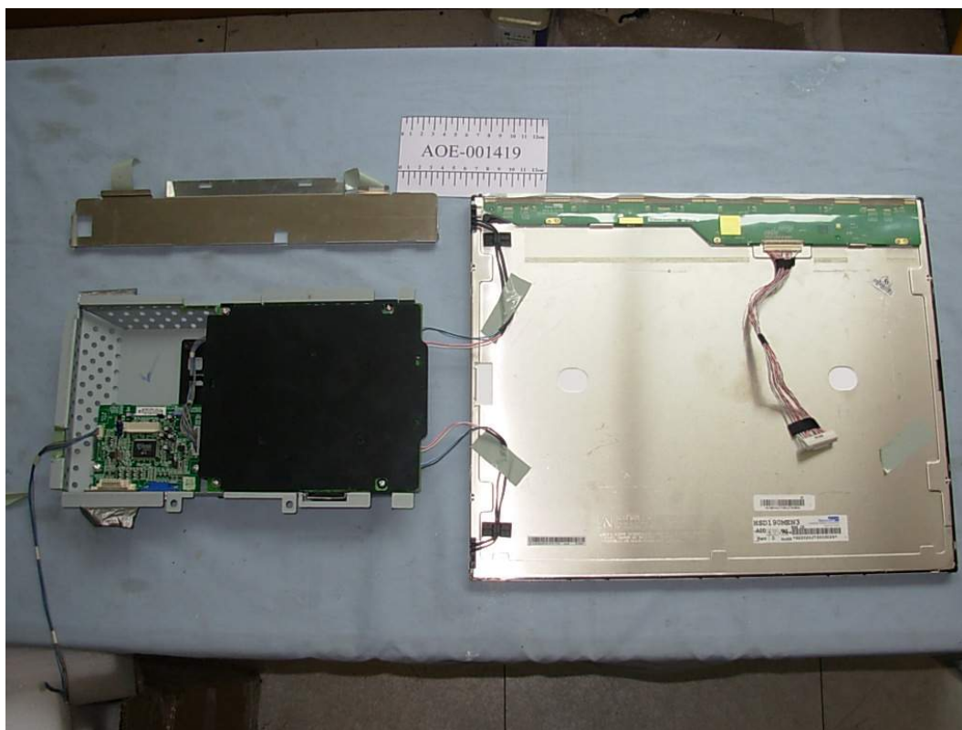
FIGURE 5 LCD MONITOR (M/N: L1954TS) BOARDS REMOVED
