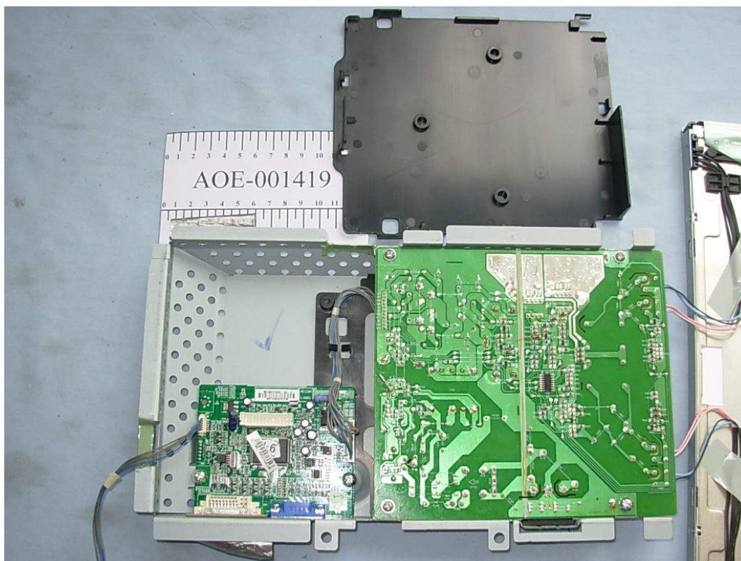
FIGURE 6 LCD MONITOR (M/N: L1954TS) BOARDS COVER REMOVED
