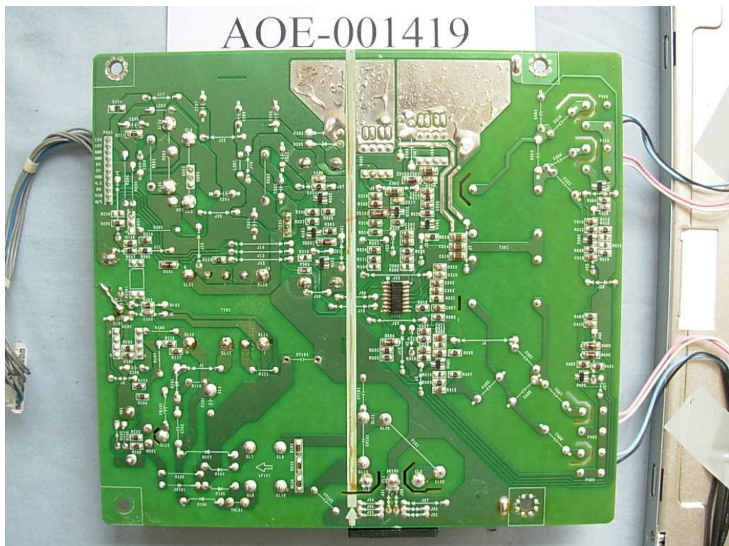
FIGURE 12 LCD MONITOR (M/N: L1954TS) POWER BOARD (SOLDERED SIDE)
