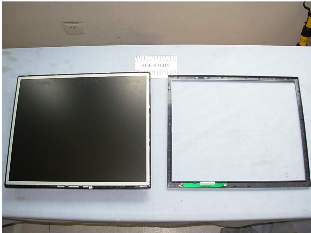
FIGURE 1 LCD MONITOR (M/N: L1954TS) FRONT FRAME REMOVED
