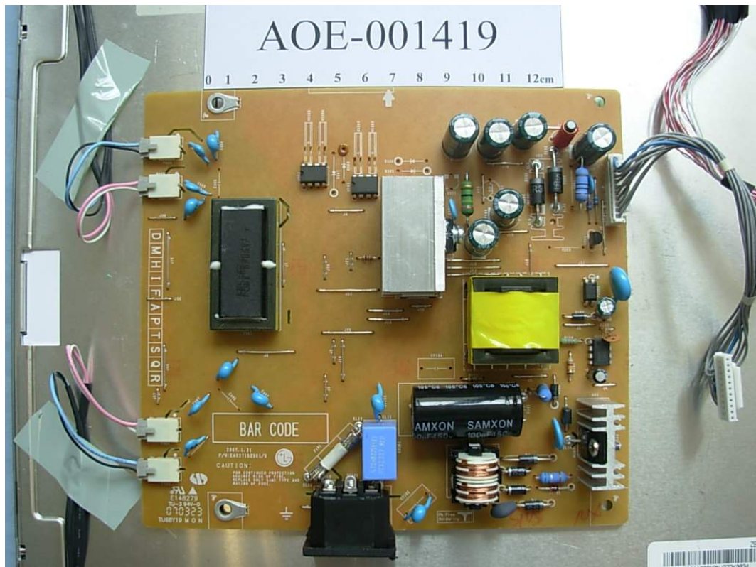
FIGURE 11 LCD MONITOR (M/N: L1954TS) POWER BOARD (COMPONENT SIDE)
