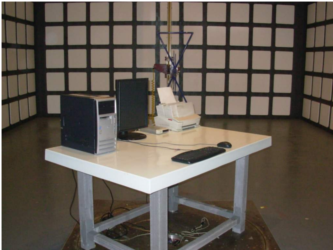
SETUP WITH MAXIMUM DETECTED EMISSION AT VERTICAL POLARIZATION (DVI 1280*1024@60Hz (ROTATE 90°))
