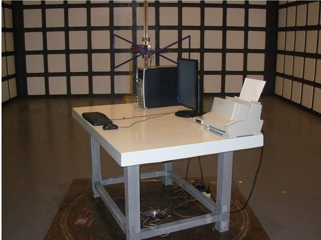
SETUP WITH MAXIMUM DETECTED EMISSION AT HORIZONTAL POLARIZATION (DVI 1280*1024@60Hz (ROTATE 90°))
