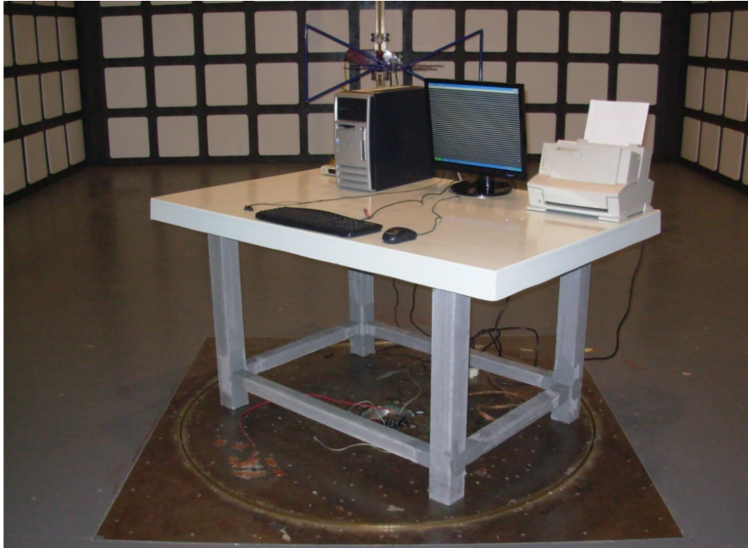
SETUP WITH MAXIMUM DETECTED EMISSION AT HORIZONTAL POLARIZATION (VGA 1280*1024@60Hz)
