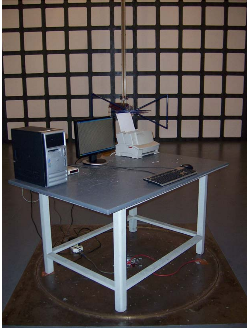
SETUP WITH MAXIMUM DETECTED EMISSION AT HORIZONTAL POLARIZATION (DVI 720*480@60Hz)
