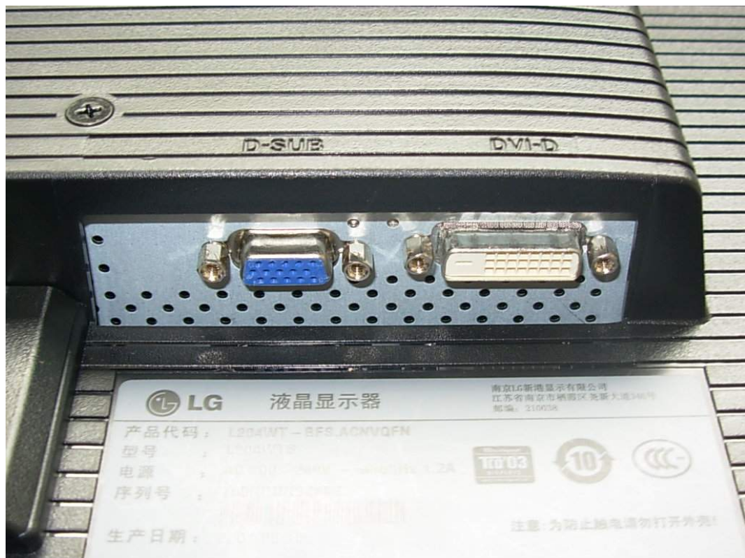
FIGURE 3 LCD MONITOR (M/N: L204WTS) PORTS
