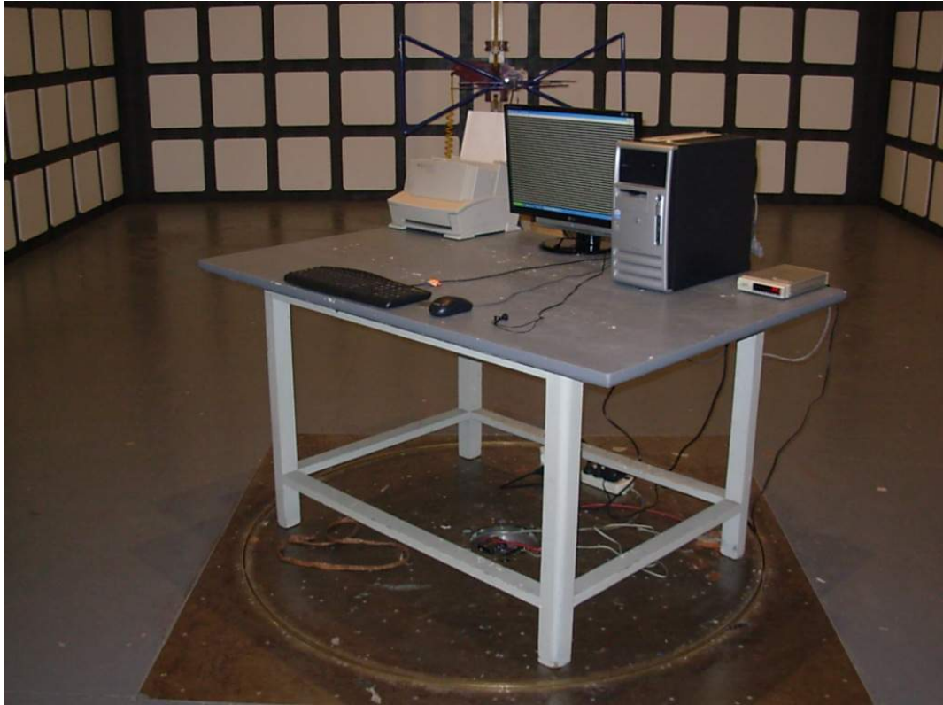
SETUP WITH MAXIMUM DETECTED EMISSION AT HORIZONTAL POLARIZATION (DVI 1680*1050@60Hz)
