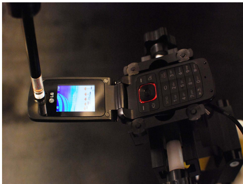
Figure 12-2 Test Setup for Wireless Device
