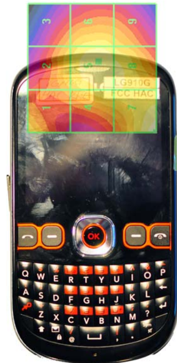
Figure 16-5 H-Field WD Scan overlay
