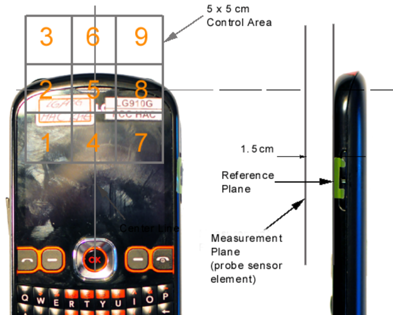
Figure 16-3 5x5 Scan grid above WD
