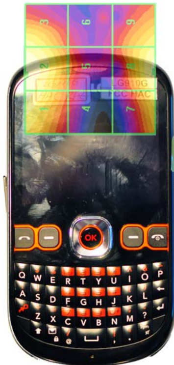
Figure 16-4 E-Field WD Scan overlay
