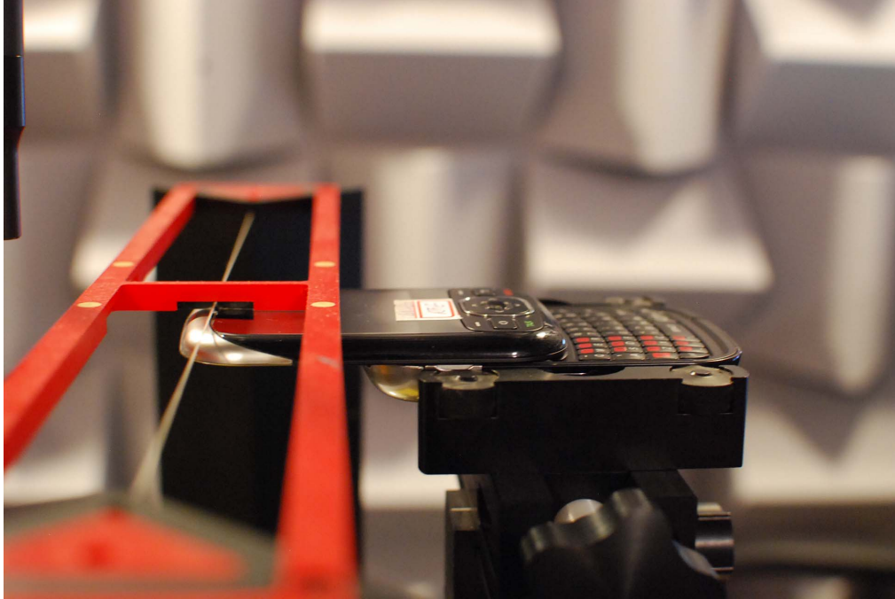
Figure 17-1 Ear Reference Point HAC Phantom Alignment
