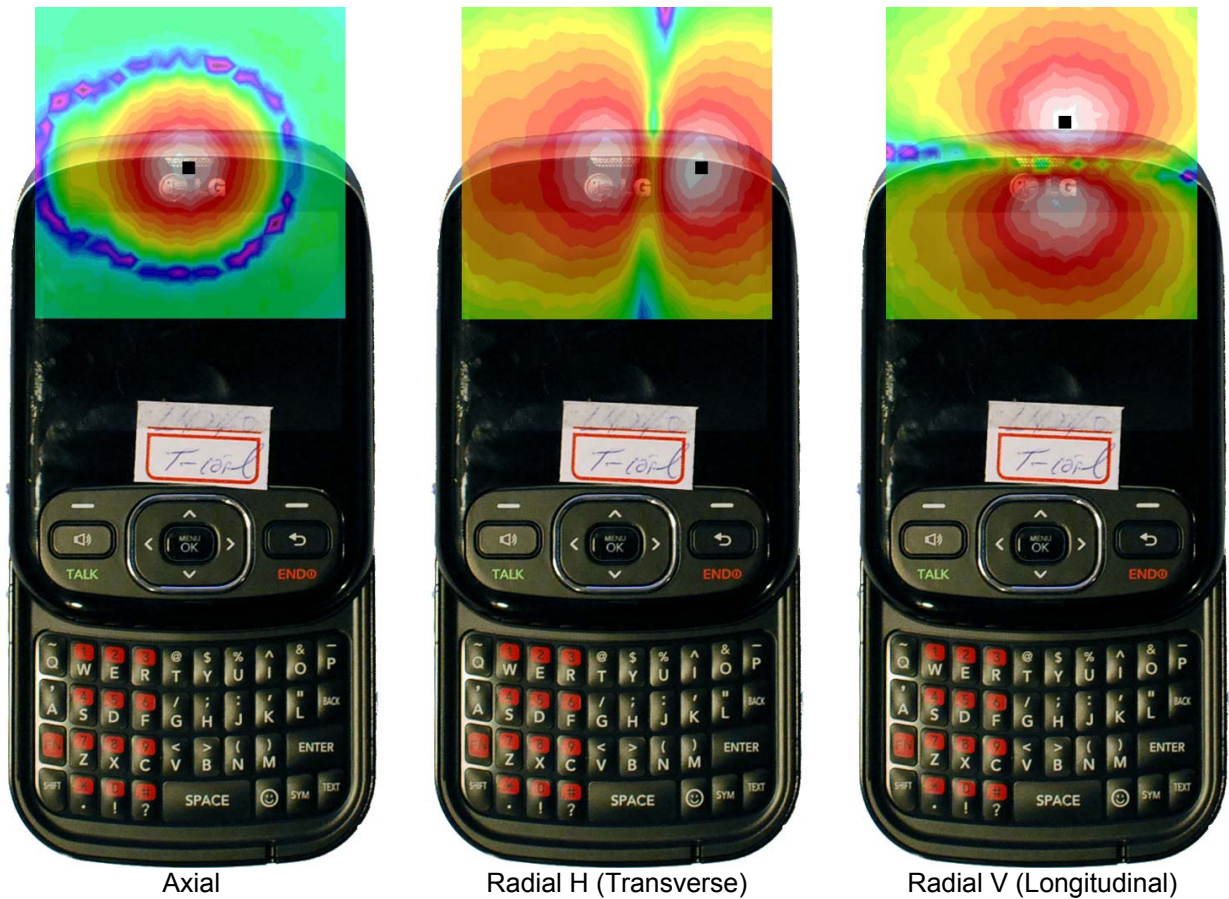
Figure 13-3 T-Coil Scan Overlay Magnetic Field Distributions
