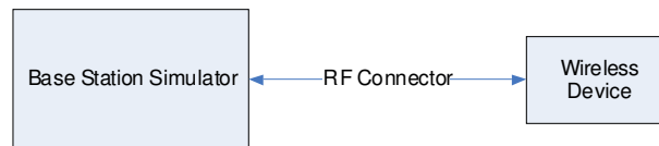
Figure 11-1 Power Measurement Setup
