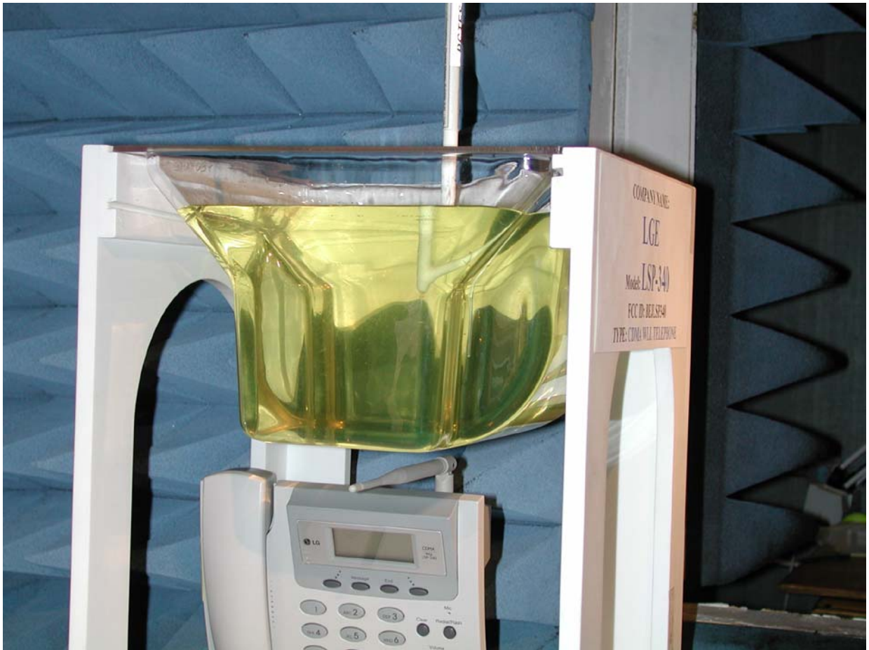
Figure 8. Test Setup of EUT in operating position with the source of significant emissions (antenna) 2.1 cm below the phantom.
