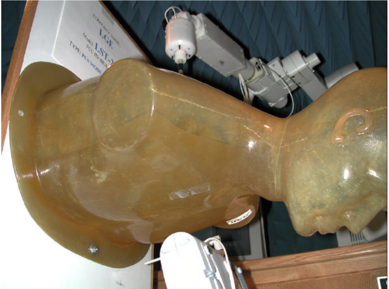
Figure 8. Test Setup of EUT in operating position with the source of significant emissions (antenna) 2.7 cm below the phantom.
