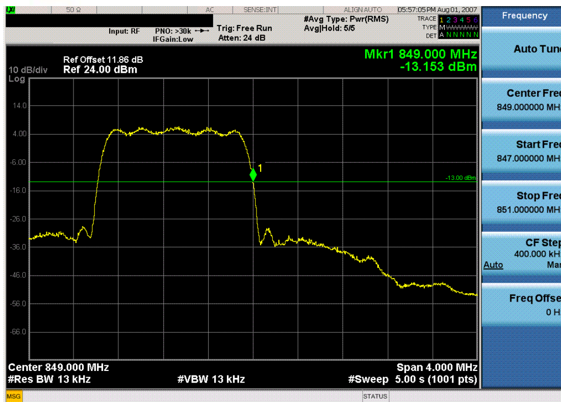
Plot 7-25. Band Edge Plot (Cellular CDMA Mode – Ch. 777)
