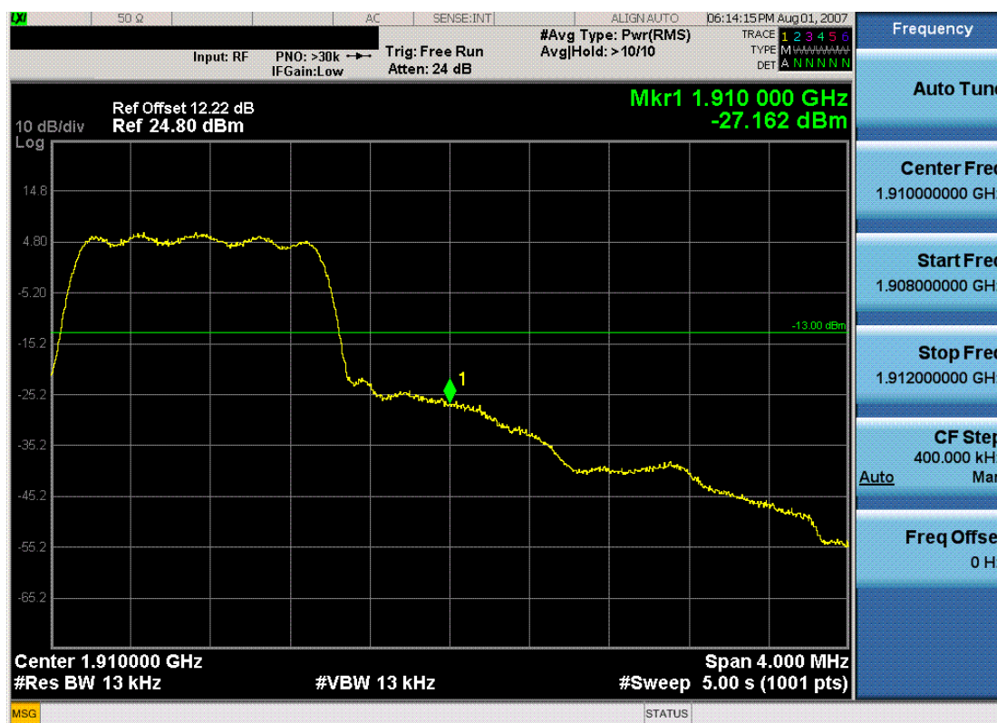
Plot 7-36. Band Edge Plot (PCS CDMA Mode – Ch. 1175)
