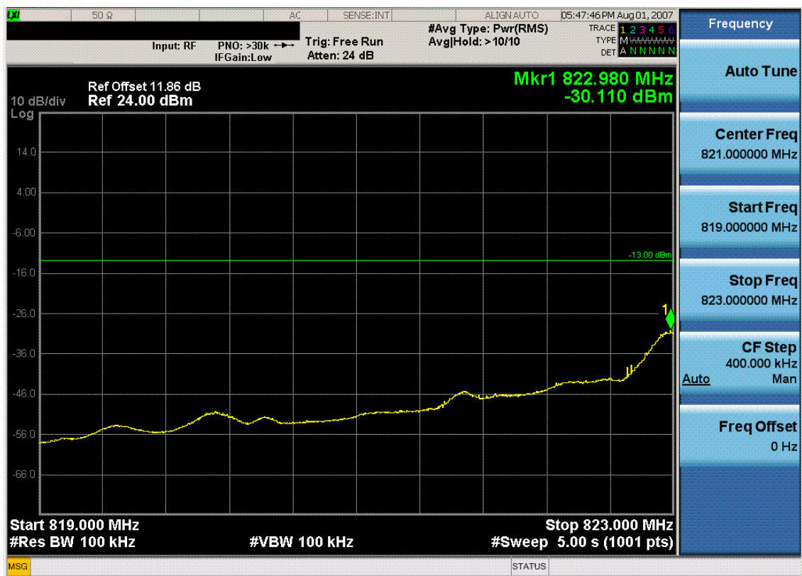
Plot 7-19. 4MHz Span Plot (Cellular CDMA Mode – Ch. 1013)
