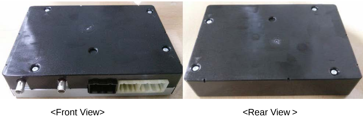
[Fig.2] VCP [module(NAD) + Power board(TCU) + Housing] setting information (Full Assembly)
