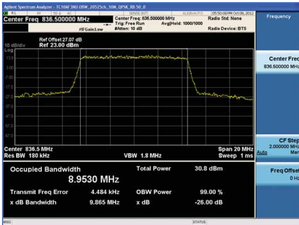
BAND 5. Occupied Bandwidth Plot (20525ch_10MHz_16-QAM_RB 50_0)
