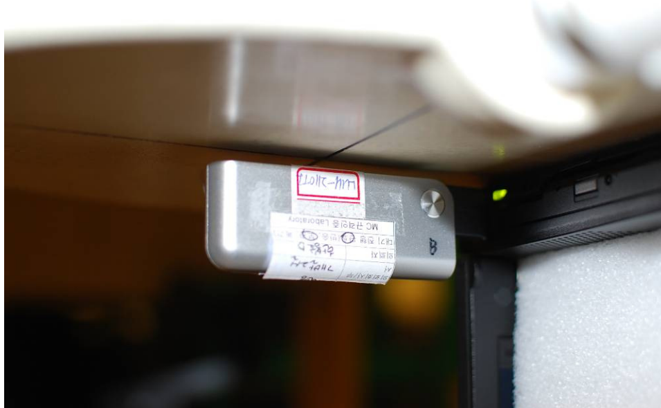
Figure 17-5 SAR Test Set Up Photo 5 Side D, Theta 180, Phi 0
