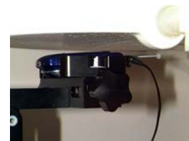
Figure 14.5 Body SAR Test Setup -- w/o Holster --
