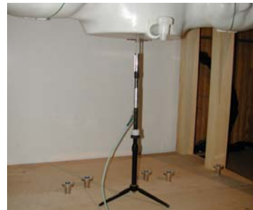
Figure 12.1 Dipole Validation Test Setup
