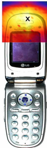
Figure 27 Sample E-field Scan Overlay
