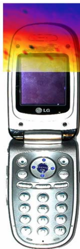
Figure 28 Sample H-field Scan Overlay
