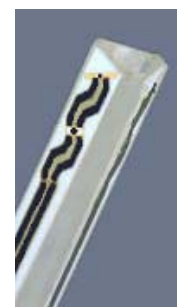
Figure 3.2 Probe Thick-Film Technique
