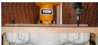
Figure 5.1 SAM Twin Phantom
