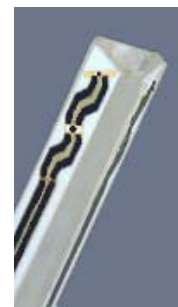
Figure 3.2 Probe Thick-Film Technique
