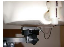
Figure 14.13 Body SAR Test Setup -- w/o Holster --
