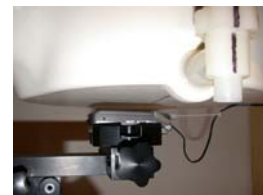
Figure 14.14 Body SAR Test Setup -- w/o Holster --
