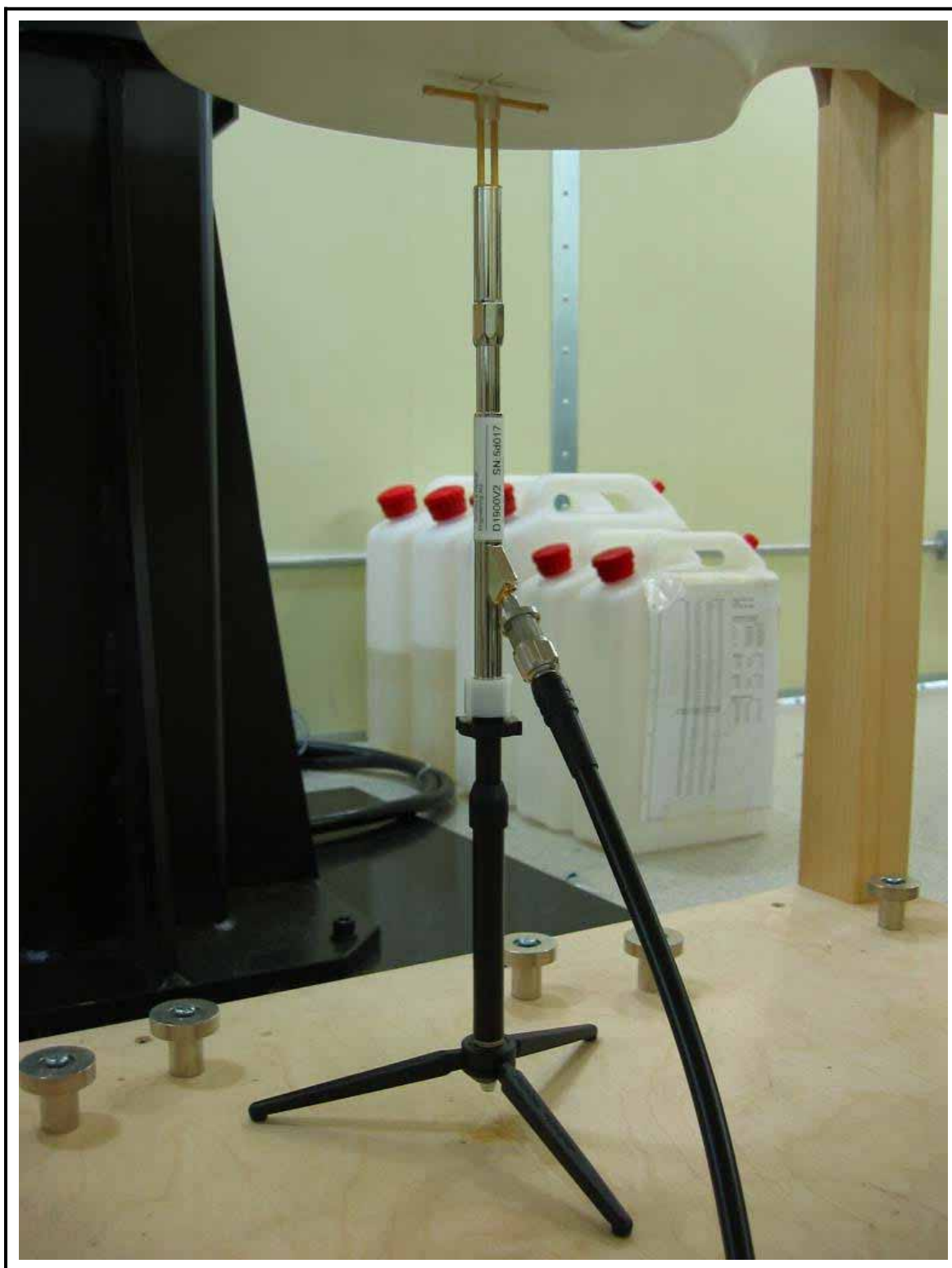
Figure 2 1900 MHz Dipole Validation Test Setup
