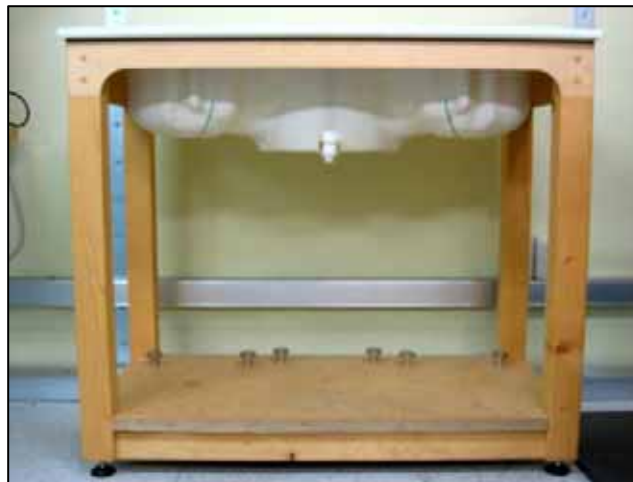
Figure 4.5 SAM Twin Phantom
