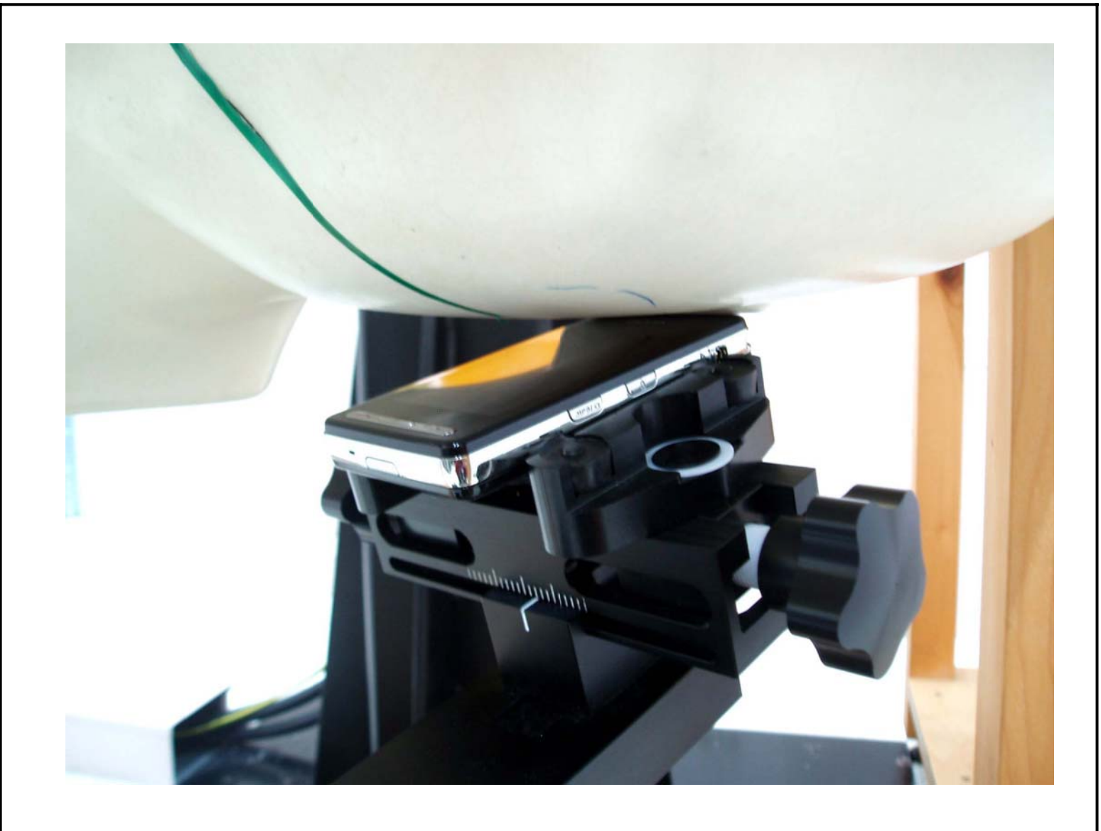
Figure 11 Left Head SAR Test Setup – Ear Tilt Position
