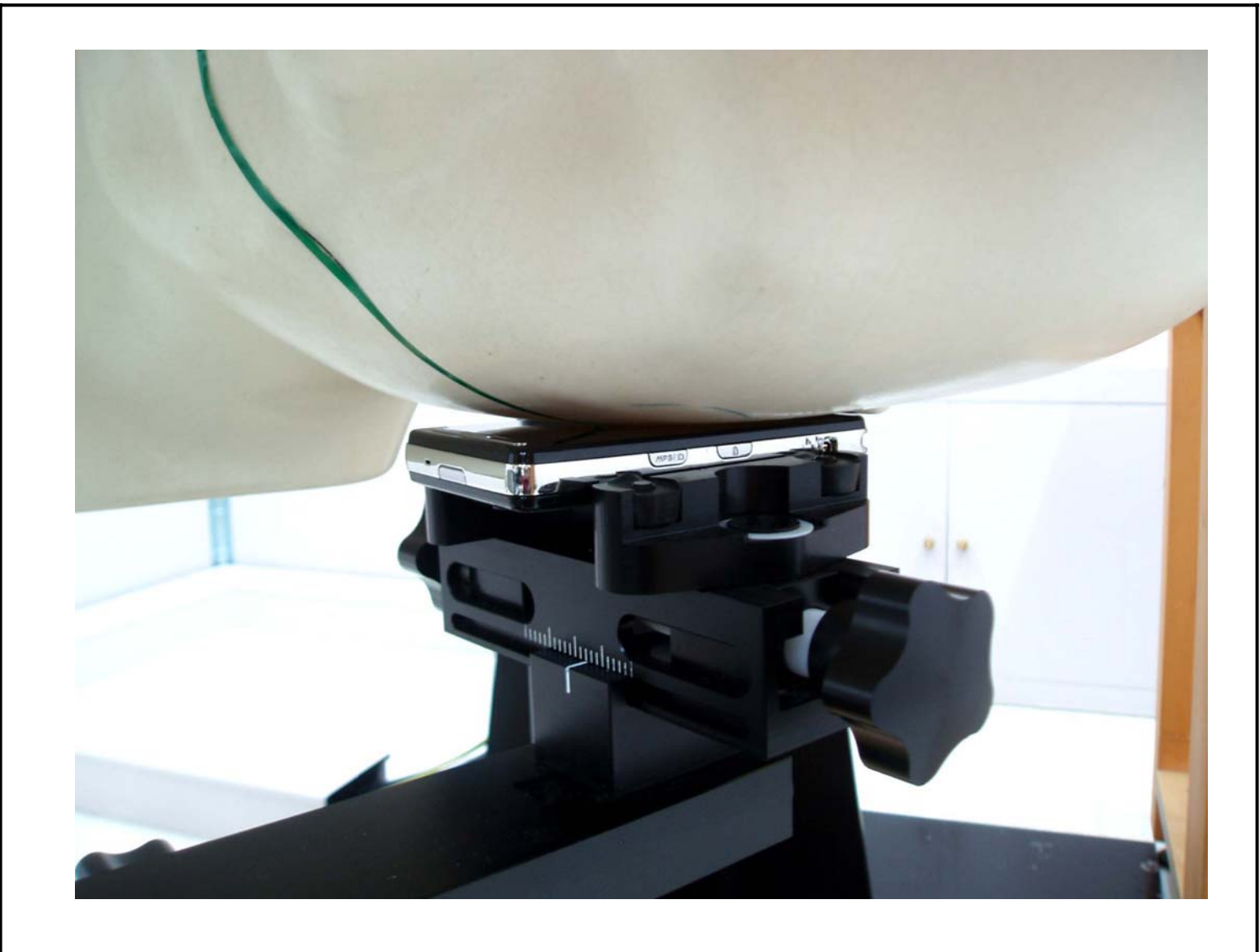
Figure 8 Left Head SAR Test Setup - Cheek Touch Position
