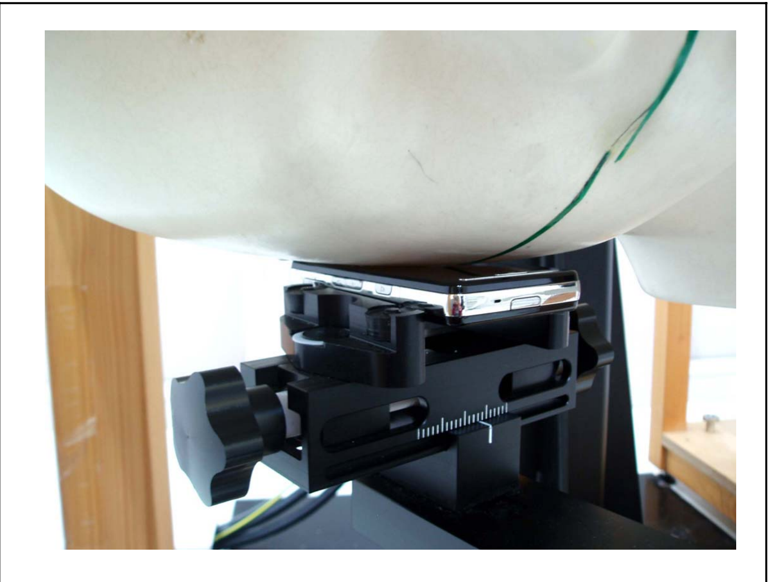
Figure 2 Right Head SAR Test Setup - Cheek Touch Position
