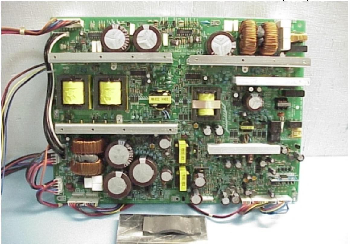
Figure 18 Power Board (Component Side)
