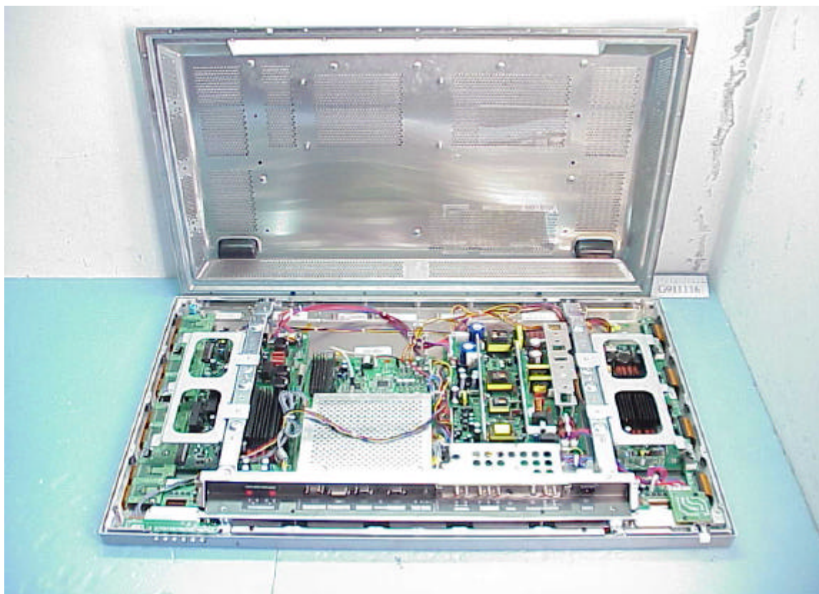
Figure 6 Internal Frame & Removed Back Cover
