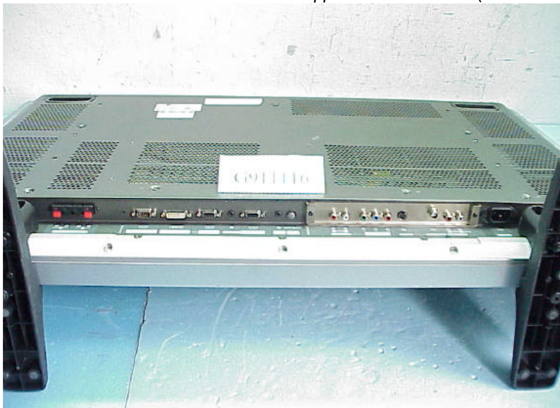
Figure 5 General Appearance/ Rear Side (I/O Connectors)
