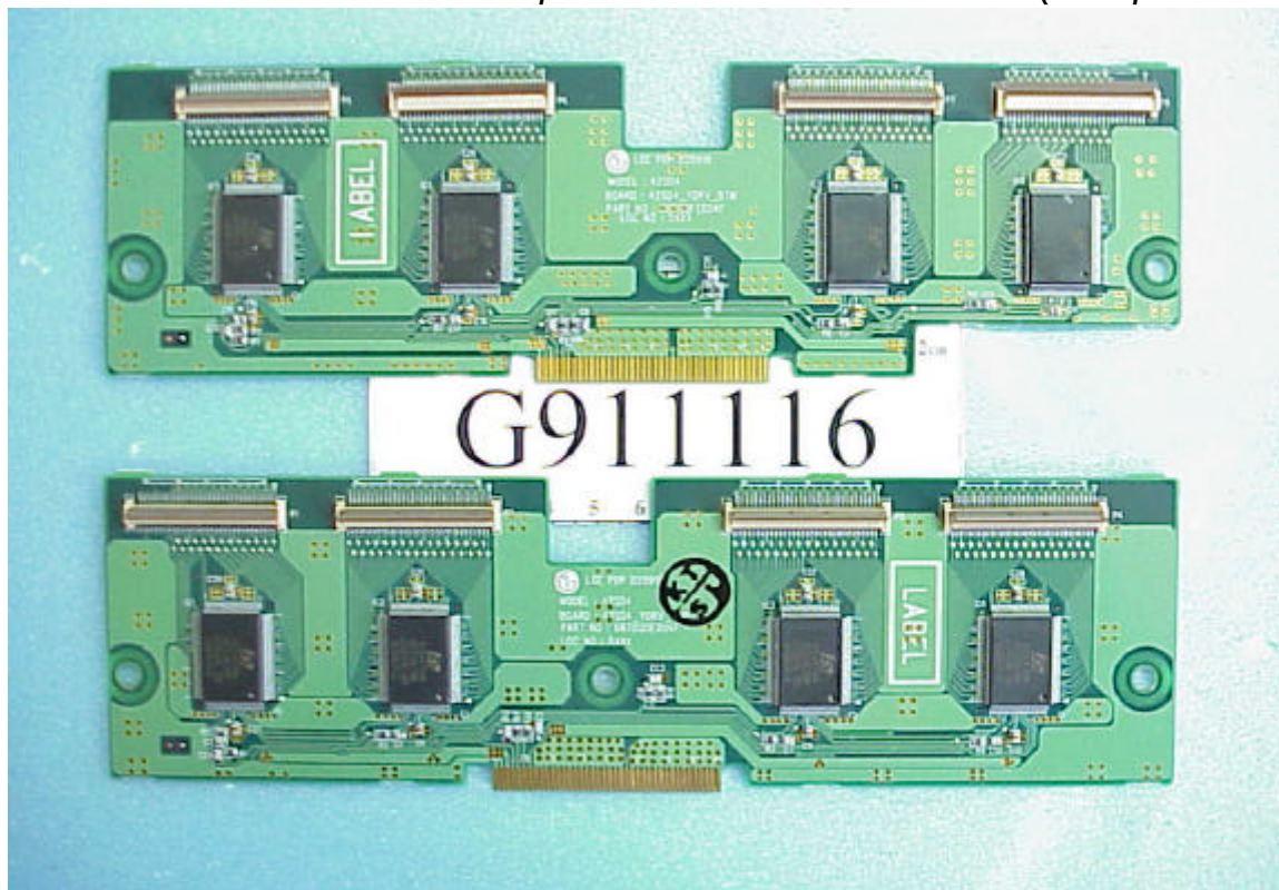
Figure 18 Y Drive Board – Top & Y Drive Board – Bottom (Component Side)
