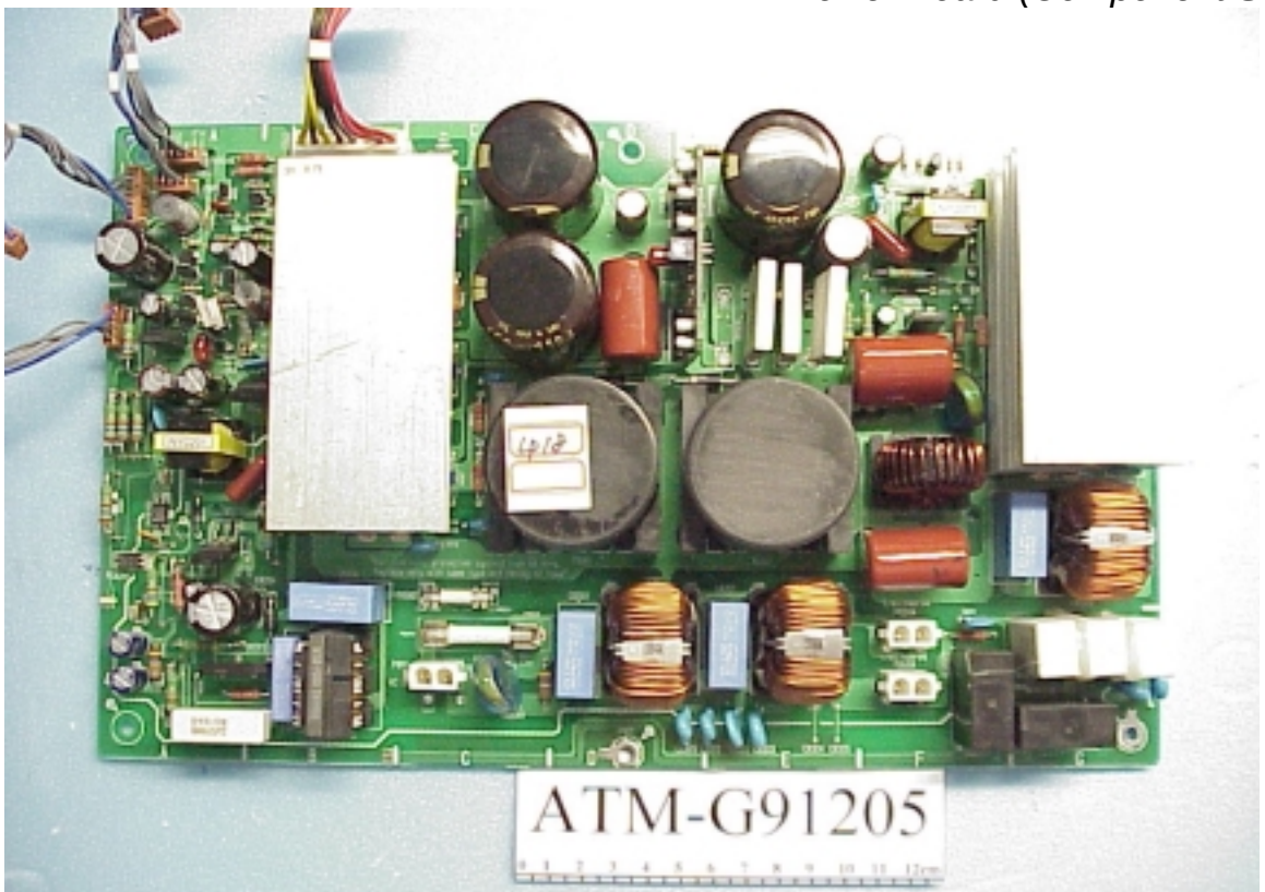
Figure 30 #2 Power Board (Component Side)
