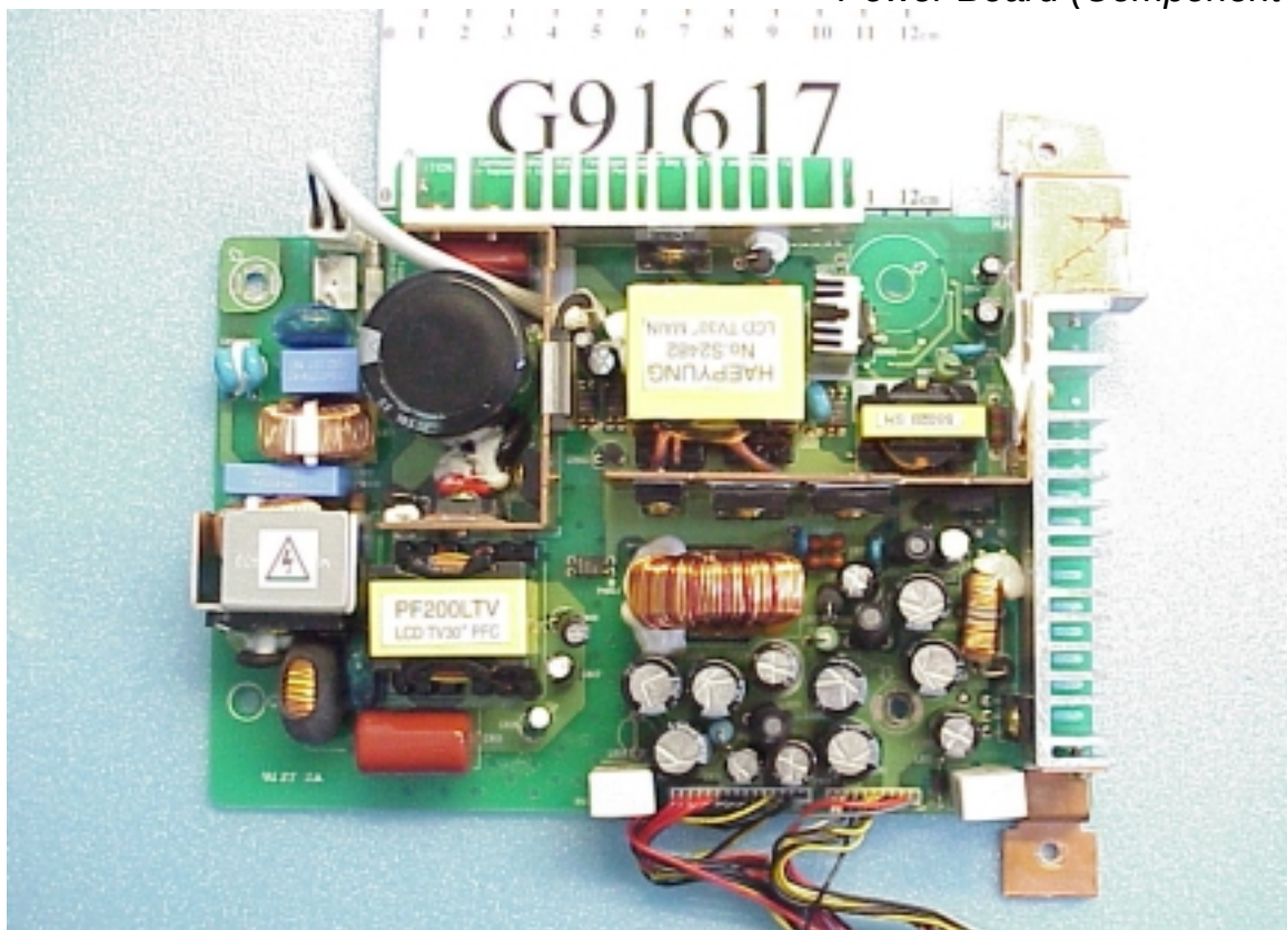
Figure 16 Power Board (Component Side)
