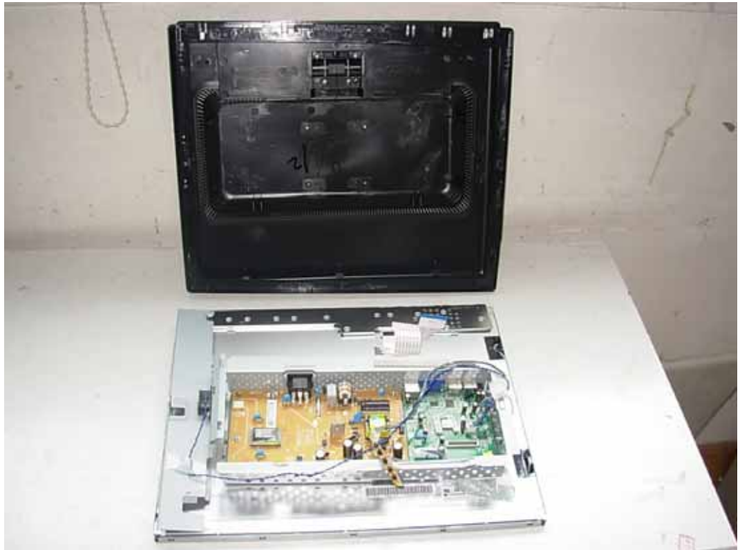
FIGURE 1 NETWORK MONITOR (M/N: N1942HET) COVER REMOVED
