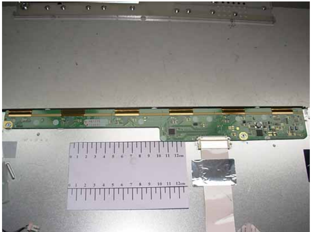
FIGURE 10 NETWORK MONITOR (M/N: N1942HET) LCD PANEL MAIN BOARD (COMPONENT SIDE)
