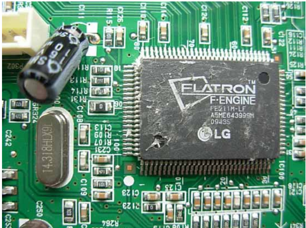
FIGURE 8 NETWORK MONITOR (M/N: N1942HET) CHIP & CRYSTAL ON MAIN BOARD
