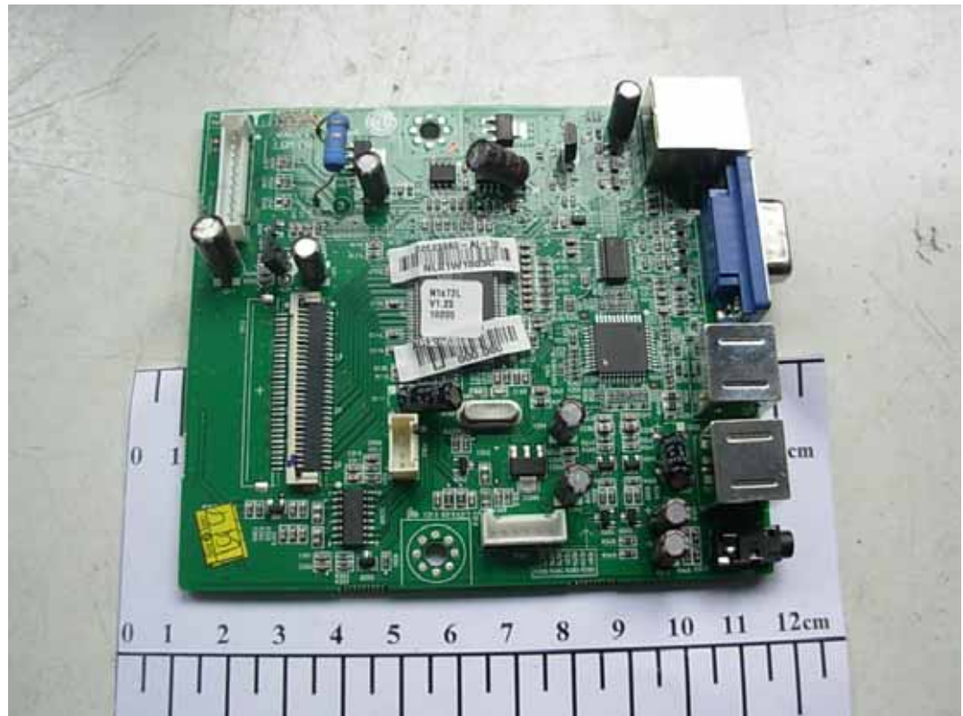
FIGURE 6 NETWORK MONITOR (M/N: N1942HET) MAIN BOARD (COMPONENT SIDE)
