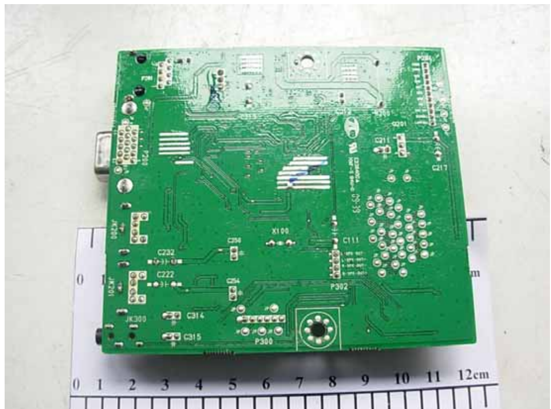
FIGURE 7 NETWORK MONITOR (M/N: N1942HET) MAIN BOARD (SOLDERED SIDE)
