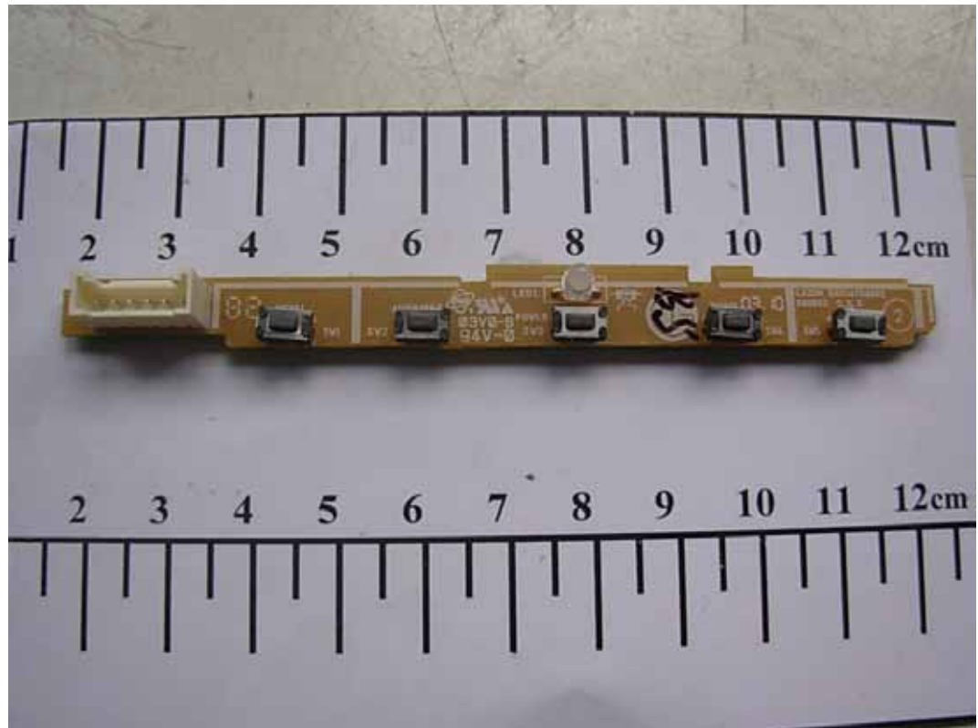
FIGURE 2 NETWORK MONITOR (M/N: N1942HET) KEY BOARD (COMPONENT SIDE)
