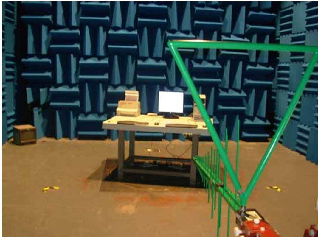
SETUP WITH MAXIMUM DETECTED EMISSION AT VERTICAL POLARIZATION (X-PORT 1440*900@60Hz)
