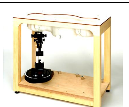
Fig 5.9 Photo of SAM Phantom
