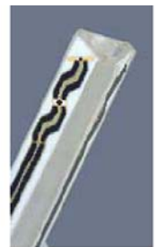
Figure 3.2 Probe Thick-Film Technique
