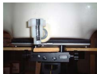
Figure 14.2 Body SAR Test Setup
