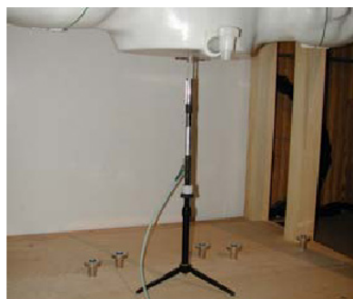
Figure 12.1 Dipole Validation Test Setup
