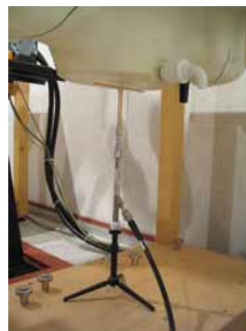
Photo of the dipole Antenna
