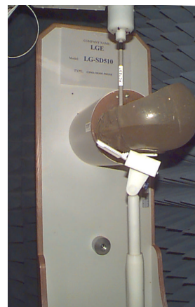
Figure 1. SAR Test Set-up
