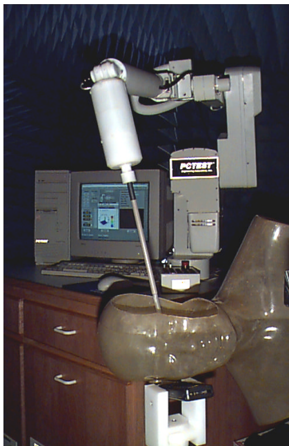
Figure 5. Photograph of the Probe and the Phantom
