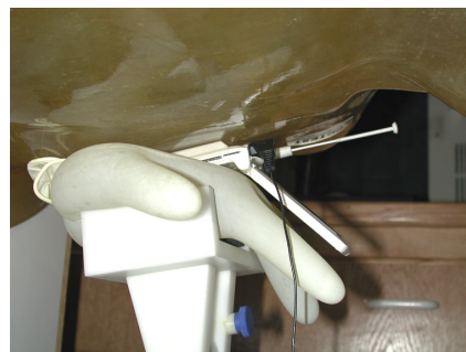
Figure 16. Hand SAR Test Setup
